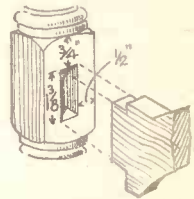
Fig. 3.—The mortise and tenon joint at the bottom of the table.
