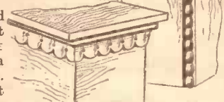
Fig. 6.—Another method in which the drop moulding is used in decoration.
