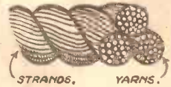
Fig. 1.—A piece of rope showing the yarns.
