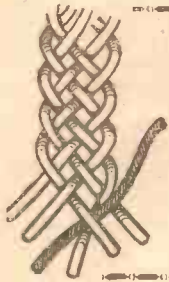
Fig. 4—How new yarns are added.
