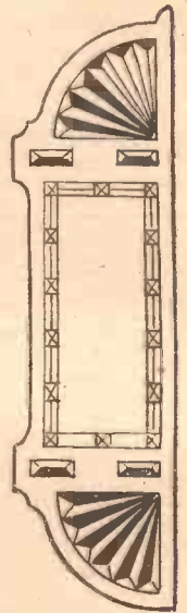
Fig. 4.—A detail of the completed carving in the sides. Note the projecting shelf tenons.
