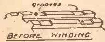
Fig. 4.—Showing how the armature windings must be bound to prevent their spreading out when rotating at high speed.
