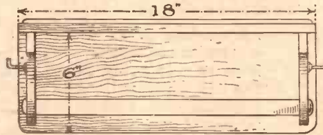
Fig. 1.—A front view with the brackets and towel rail in position. Measurements of the back are also given. Note the beading on the shelf to prevent bottles sliding forward.
