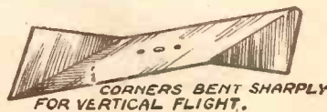
A piece of tin should be cut to the above dimensions and bent according to the flight required.
