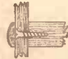
Fig. 3.—A section showing how the towel rail is fixed and the head of the screw covered.
