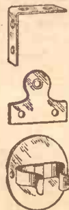
Fig. 2.—Three useful fittings supplied by Hobbies Ltd. The top one is an angle plate, the centre one a hanger, and the lower one a tool clip.
