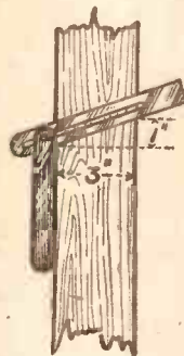
Fig. 2.—Marking the angle on the side pieces.
