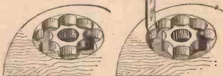
Fig. 2.—The first illustration is of hole drilled to make a large recess, the shoulders being cleaned away as shown in the second picture
