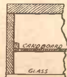
Fig. 2—A sectional view of the box for holding the sand.
