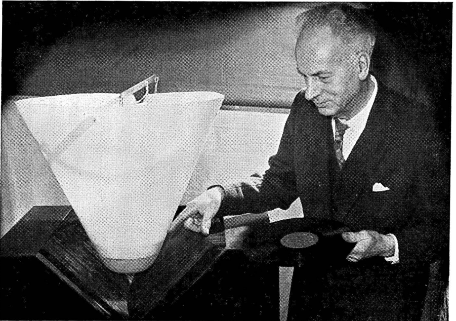
The author demonstrates his giant model which simulates stylus behaviour on a scale of about X 5000! When the groove moves under the tip, the stylus "goes into orbit", as lateral and stereo conditions are created.
