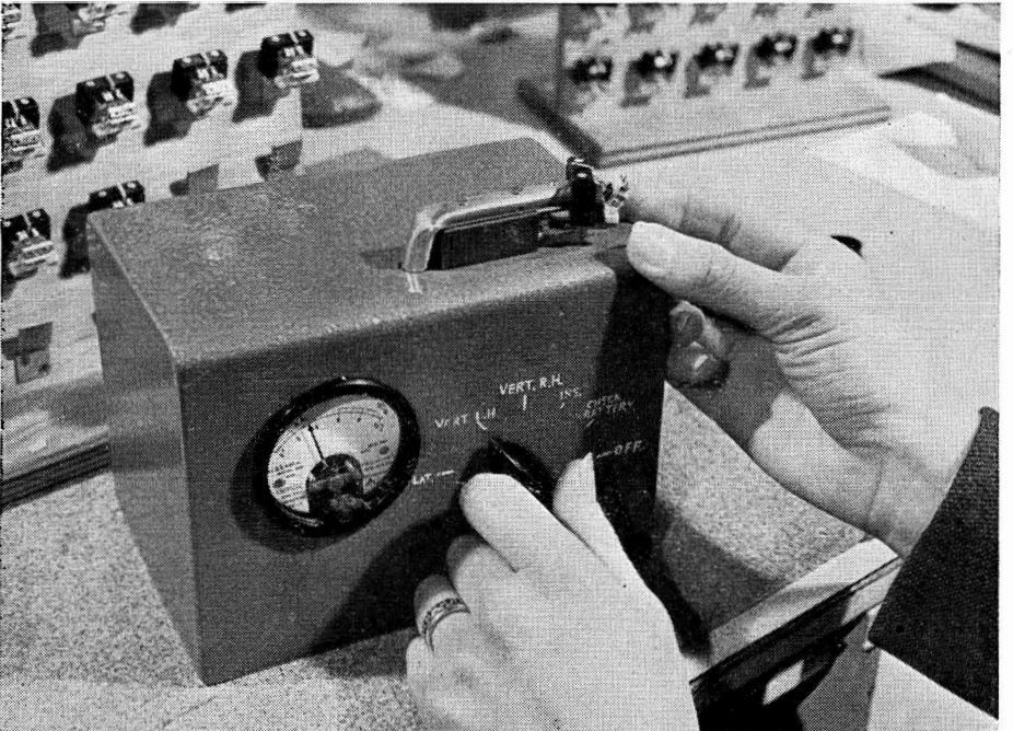
13. This instrument tests the insulation and electrical continuity of the complete head.
