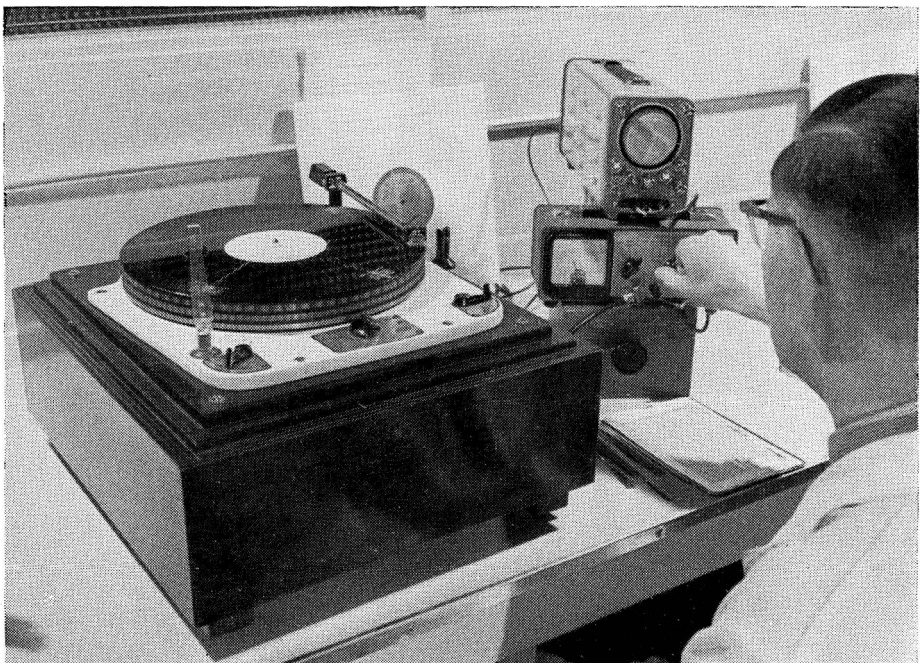
15. Final tests. With C.R.O. and meter the output from a test disc is measured.
