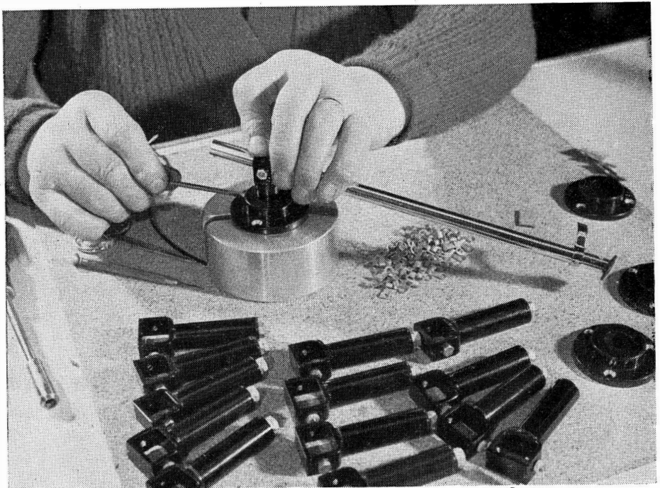
11. Final stages of arm assembly include the fitting of pillar and mounting flange.
