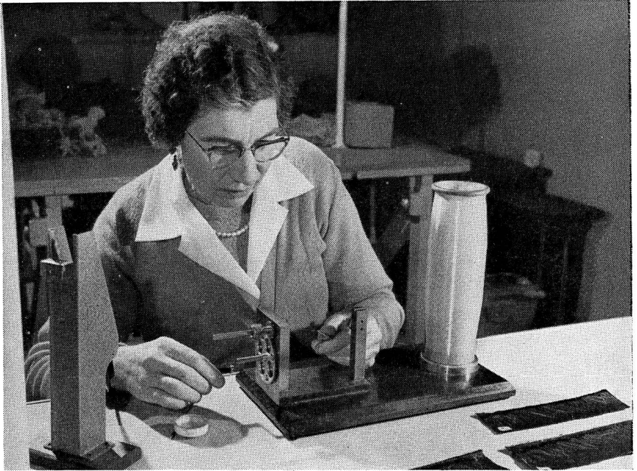
1. Tie-back loop of fine Terylene to prevent forward stylus movement.
