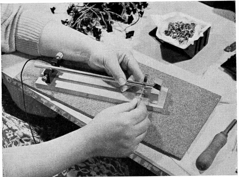
10. Here, the wire is inserted, the contact plate added, and the lifting handle fitted.
