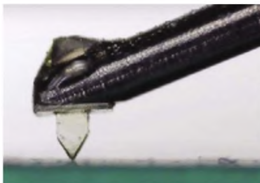
Wally tools picture an upright stylus in what appears to be a boron rod, adhesively bonded into place on a surface ground flat.
