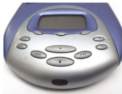
The DAP Jukebox was controlled via this intimidating collection of controls, which include three function-dependent 'smart buttons' under the screen. Unfortunately, the user interface was rather clumsy and unresponsive. Apple was to change the game a year after the DAP Jukebox's launch, with the user-friendlier iPod.
