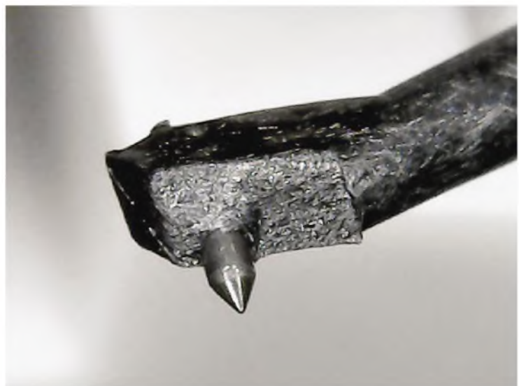
This picture shows the fibrous nature of the cantilever and what appears to be a ground-on flat to accept the stylus shank.
