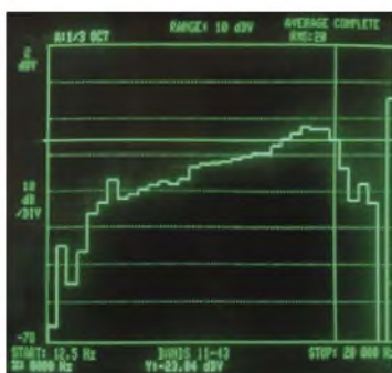
A third-octave analysis of pink noise from the LS-55's preamp output shows treble dominance. The cursor is at 8kHz.
