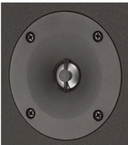
The titanium dome tweeter has a frontal phase plate to flatten its frequency response by suppressing cavitation at the dome's apex. It sits in a shallow horn that directs energy forward.
