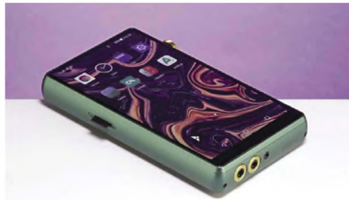
Two 3.5mm stereo jacks (gold) sit at the bottom of the case, with a tiny 2.5mm balanced outlet (black) alongside. The microSD card pops into a spring loaded slot.
