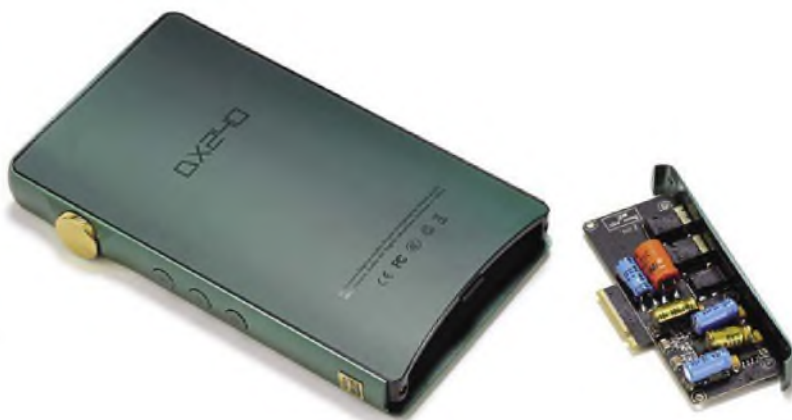
The AMP module slides out from below, after two miniature Torx T5 screws are removed. Other modules are available, AMP8 proving a better balanced output.
