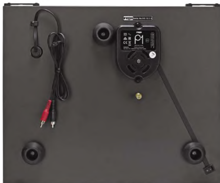
Underneath the P1. Three solid rubber feet, an arm lead with no separate earth and a 24V a.c. synchronous motor fed by an external wall wart. The low voltage supply and non-metallic plinth remove a need to mains earth, avoiding a hum loop.
