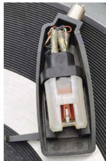
Decca Deram ceramic cartridge. "Arguably the best ceramic cartridge ever produced and claimed to be of transcription quality" says Alan Scott.
