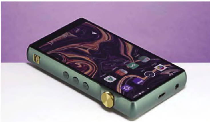
A large rotary volume control worked smoothly. At top is a USB-C socket for charging/computer connection, as well as an electrical S/PDIF 3.5mm digital output jack.
