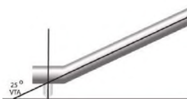
Our diagram shows the most common situation where an alloy tube's crimped end is bent to suit upright stylus fixing.
