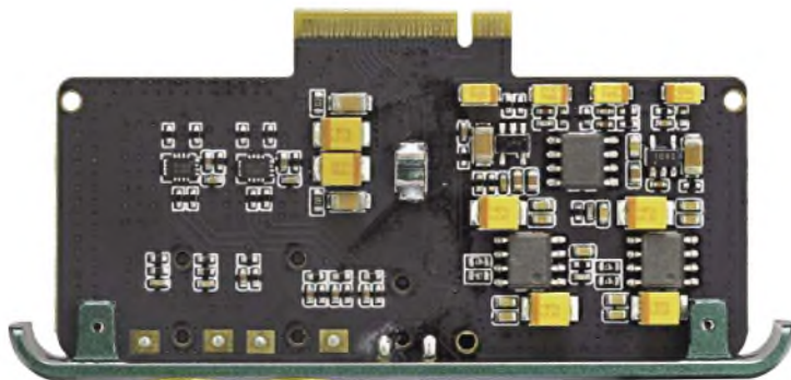
The AMP1 Mk3 output amplifier uses surface-mount mini components, including three chip op-amps at right.
