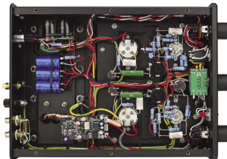
The unit is hard-wired with sturdy discrete components. At low left lies a screened Bluetooth receiver and DAC board.
