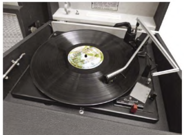
Fitted to the Gondolier is a Garrard 2025TC – a changer of higher-quality than that fitted to cheaper record players. Also available, for an extra £2 12s, was a version optimised for 'manual' playback of records using the classic Garrard SP25.
