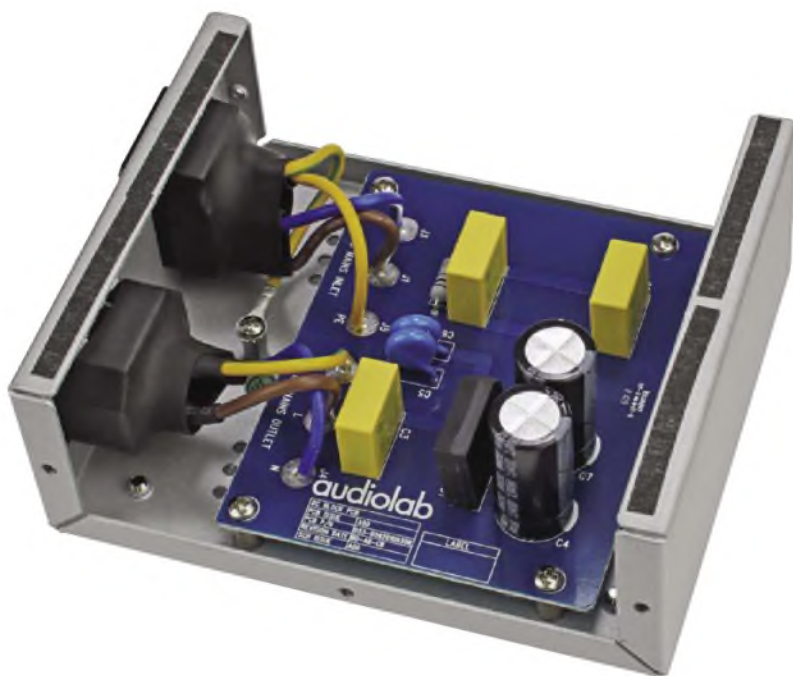
A fairly simple circuit board with two high voltage electrolytic capacitors of 10,000µF apiece Audiolab say, plus filter components.
