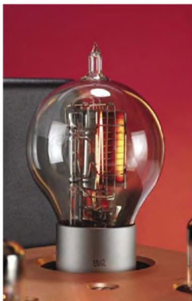
The open electrode assembly of a 205D valve makes its glowing heater obvious. A visual treat from 1924.
