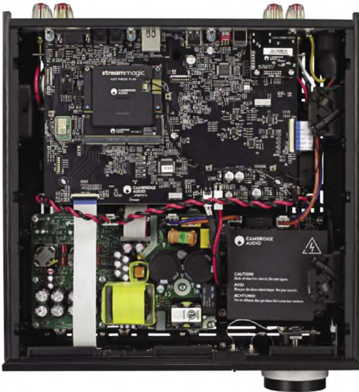
A deeply complex interior of densely packed surface-mount components. At bottom centre is the switch-mode power supply, above it their StreamMagic module.
