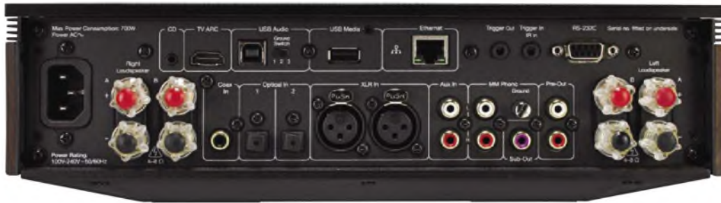
Two pairs of loudspeakers can be connected to conventional terminals (at left and right). USB B socket and RJ45 ethernet socket are rare partners (top centre). Between them lies a USB A socket for 'mass storage' devices (Flash Drive).
