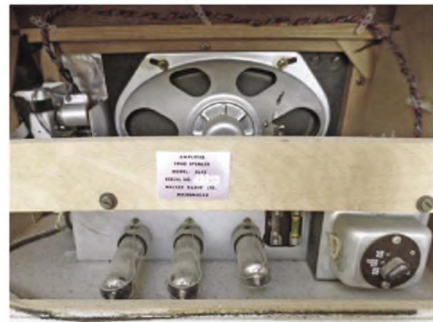
The AL42 'amplifier loudspeaker unit' contains the same chassis and Goodmans 15 Ohm 10in. x 6in. elliptical speaker used inside the Gondolier.
