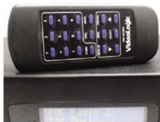
The remote control accesses some functions that cannot be invoked via the front panel – among them nine 'presets' of favourite stations. However, some are DAB+ and cannot be received by the DRX-601E.
