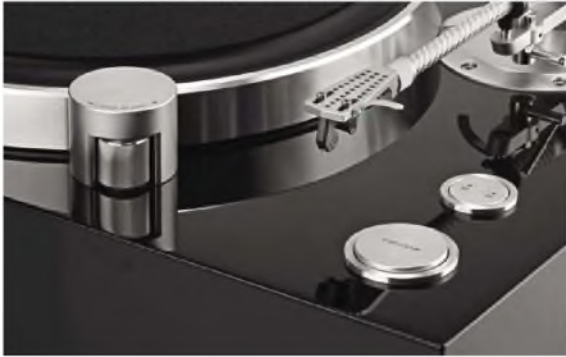
The plinth pillar (left) carries a knurled speed adjustment roller that moves in click-steps. At right a start/stop button and 33/45rpm button with small green LEDs to indicate speed-lock.
