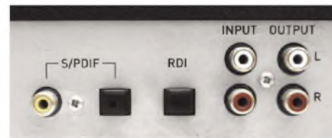
The audio input accommodates an external analogue tuner; the DRX-601E is digital-only. The optical RDI (Receiver Data Interface) carries the raw multiplex bitstream but no compatible add-ons were ever marketed.
