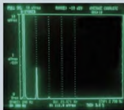
Distortion (3.2%) due to tracking error. Second harmonic only.
