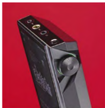
The volume control has an illuminated bezel that changes colour according to mode.
