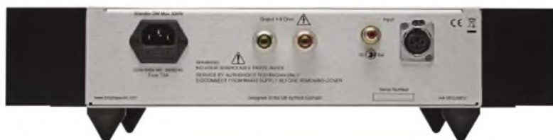
A neat rear panel with IEC mains input at left, one pair of sturdy gold plated loudspeaker sockets and, at right, phono socket and XLR inputs.
