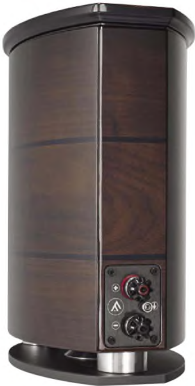
The F1-5's cabinet has a furniture-standard finish and is attached to a heavyweight machined aluminium plinth. Adjacent to the gold-plated speaker terminals is an earth terminal that grounds the driver chassis to avoid radio frequency interference.
