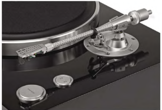
Yamaha's unusual straight tonearm. With no angular offset of headshell and cartridge, bias correction is unnecessary. A manual lift/lower lever is fitted for cueing. There are no auto-systems.
