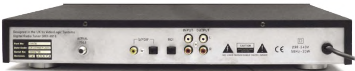
An 'F' socket accepts the VHF Band III (174-230MHz) DAB radio signals from the aerial. As well as the analogue outputs (and inputs), digital audio is available in both optical and coaxial form, to feed an external DAC.
