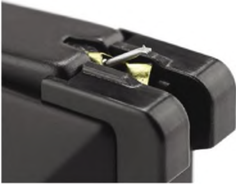
The cantilever uses a parallel sided aluminium tube with, Sumiko say, a line contact stylus attached direct (nude). The stylus assembly can be removed for replacement.
