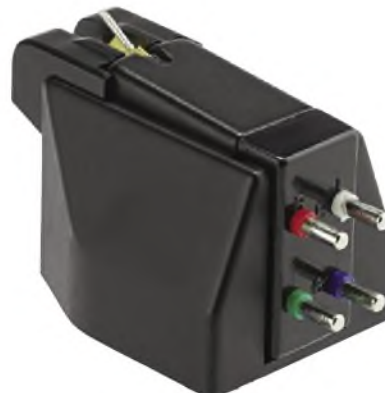
At rear lie conventional connecting pins, right channel being red (+) and green, left channel white (+) and blue.
