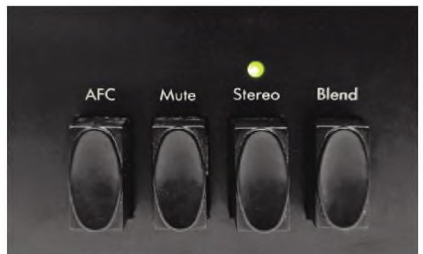
The push-button controls are AFC (automatic frequency control) to prevent drift, Mute to kill noise between stations, Stereo/mono – the latter for weak stations, and Blend to reduce hiss on stereo.
