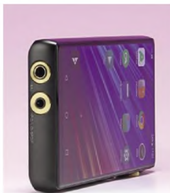
Underneath lie a 4.4mm balanced output jack (top) and conventional 3.5mm stereo jack.
