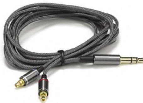
The proprietary colour-coded 'locking' connectors of the supplied lead mate with similarly gold-plated receptacles on the buds; a standard 3.5mm stereo jack plug terminates the other end.
