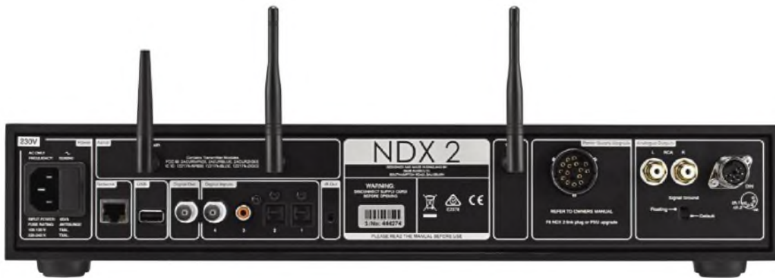
Two external wi-fi aerials and one Bluetooth aerial help make the NDX 2 sensitive to household router and phone signals, aiding data speeds and reception stability. There is an array of digital inputs and Naim's DIN socket output at right, but no XLR balanced outputs from the DAC.
