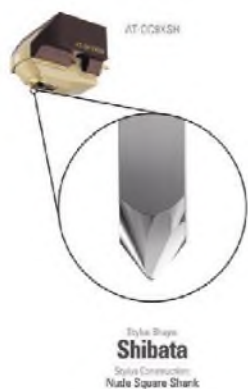
Audio Technica's diagram of the 1970s Shibata (SH) stylus, illustrating its profile with multiple face grinds. Use this for CD-4 LPs!
