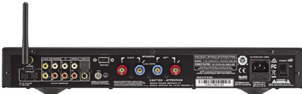
The rear of the NAD includes a Bluetooth aerial as well as digital and analogue inputs.
