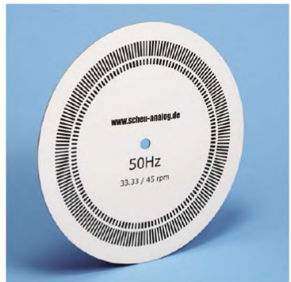
A classic strobe disc from Scheu Analog, supplied with their Cello Classic turntable. It has 182 bars (outside) that should appear stationary when lit by a 50Hz powered light bulb (old fashioned sort).
