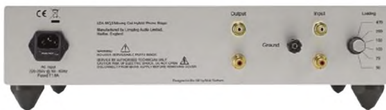
Rear panel carries IEC mains input socket, gold plated phono sockets and a rotary switch to adjust load.
