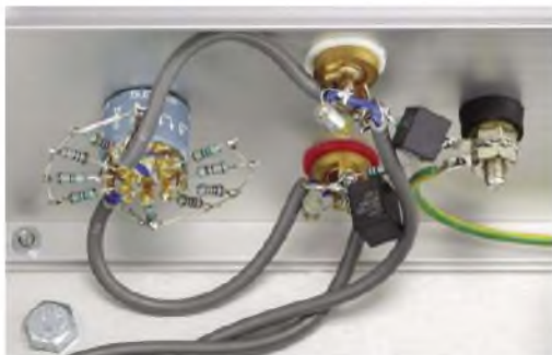
The load switch, at left, switches resistors across the input.
