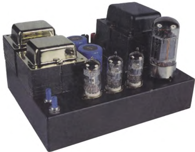
The World Audio Design 4 Watt amplifier designed by Tim De Paravicini – and very popular in its time. "What matters is not so much an amp's absolute power as its ability to deliver it" notes Aaron Proctor.
