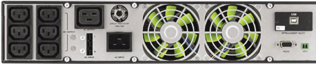
The rear panel carries six IEC power outlets, plus a high current outlet for a 13A mains block. Also, there are two cooling fans, an overload re-set switch and computer monitoring outlets (right).
