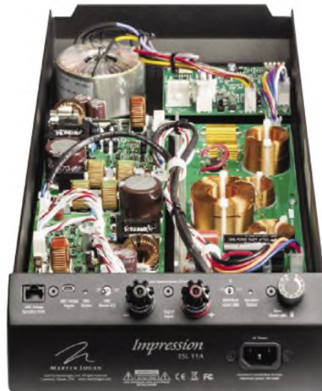
Big crossover section at right, twin Class D power amps, Digital section and linear power supply all sit in the base tray.
