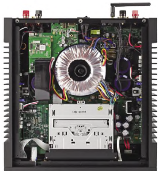
Inside is a linear power supply based around a large toroidal transformer, plus Class A/B power amps at left and right, attached to their heatsinks. At bottom (in the pic) is the auto-load (no tray) CD drive.
