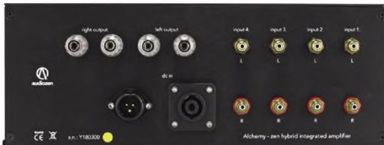
The rear panel of the Audiozen amplifier main unit has four analogue inputs (right) plus the two captive power supply sockets at the bottom.
