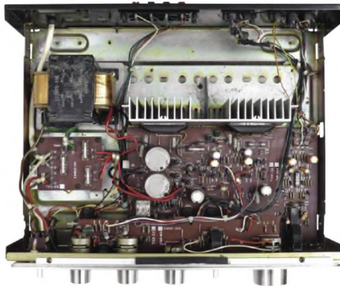
Construction and design of the JVC JA-S11 is fairly typical of 1970s mass-market Japanese hi-fi gear. Its power amplifiers use Sanken S-40W 'hybrid Darlington modules'. Rear internal metal work is cadmium (passivated) plated – now viewed as toxic – so beware.
