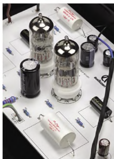
E88CC valves are employed for the pre-amp section. Audiozen sources new old stock (NOS) tubes for this.
