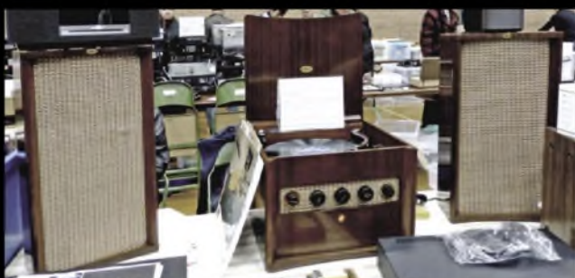
A UK-made Capitol/EMI RS101B circa 1959. One of the first stereo players on the market, the RS101B featured off-board speakers to help the listener achieve a decent image. Turntable is a four-speed Garrard. This lovingly-restored example was supplied with two cartridges – mono and stereo. Your £400 also bought a spare turntable.
