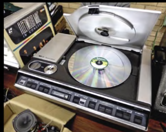
A mint-condition Philips Laservision player where an LP-sized analogue disc was scanned by a Siemens helium-neon laser. £100 would have secured you this museum piece, which will even work with modern flat-panel TVs provided they have analogue video inputs. A pair of phono sockets allow analogue audio to be fed into a hi-fi system.
