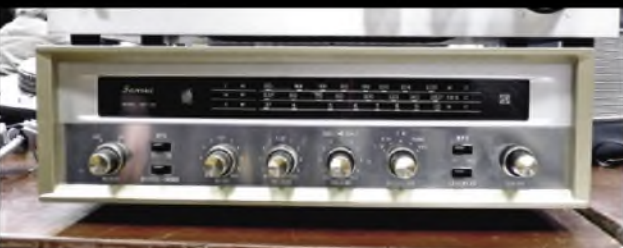
A Sansui SM-12M low-power (4 watts) receiver, circa 1961. There's not only short-wave coverage but a 'magic eye' tuning-indicator. For the £100 asked, a great intro to the 'tube sound'; efficient speakers are a must here!
