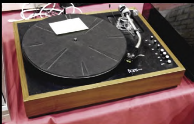
A UK-made Capitol/EMI RS101B circa 1959. One of the first stereo players on the market, the RS101B featured off-board speakers to help the listener achieve a decent image. Turntable is a four-speed Garrard. This lovingly-restored example was supplied with two cartridges – mono and stereo. Your £400 also bought a spare turntable.
