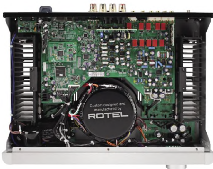
A massive toroidal mains transformer accounts for much of the amplifier's weight. Large heatsinks at left and right keep the output transistors cool. Small-signal sealed relays provide switching.
