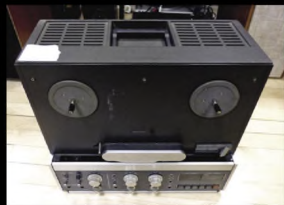
The owner of this complete Revox B77, a fairly standard half-track model with 9.5cm/s and 19cm/s speeds, was letting it go for a mere £50 – one of the biggest bargains of the show! It was sold as 'spares or repair', but its heads seemed to have plenty of life in them. One of its flimsy toggle switches had snapped off.
