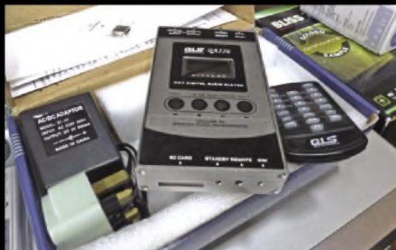
A QLS QA550 from China – an unusual solid-state media player intended to replace a CD transport. Using SD cards, it's optimised for 16-bit/44.1kHz WAV files 'ripped' from CDs, having no analogue audio outputs. Instead, its S/PDIF digital output feeds an external DAC. This 'upgraded' one, boxed and complete with remote control, was £40.
