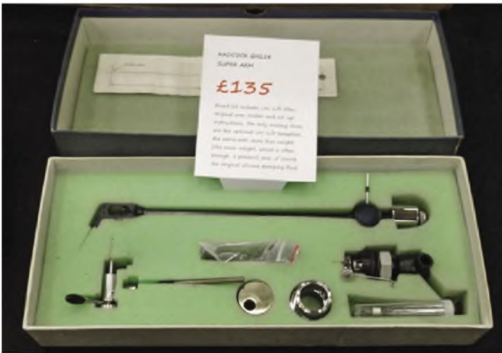
Hadcock GH228 unipivot arm – difficult to handle on a bouncy suspended turntable.
