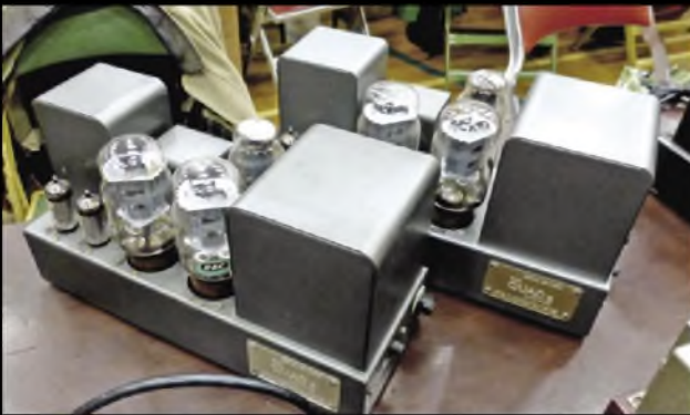
A pair of Quad II valve power amplifiers (15 Watts) – valued classics. These were unrestored and being offered for £700. They need a Quad 22 pre-amplifier however (or home built equivalent!).
