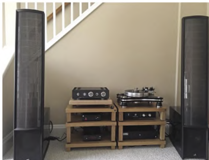
Martin Logan Classic ESL9 hybrid electrostatic loudspeakers 'at home' in New York. Best driven by a Sugden A21SE (top left) says John Speight.
