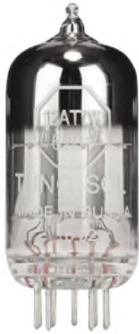
Two Tung-Sol 12AT7 (ECC81) double triodes are used to drive the HEXFET output stage of each channel.
