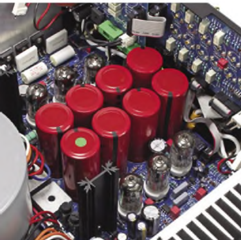
Russian-made Tung-Sol 12AX7 valves (ECC83) perform input duties, and 12AT7s (ECC81) lie in the driver stage. Also visible are red power supply smoothing capacitors, the heatsinked output HEXFETs and miniature signal relays.
