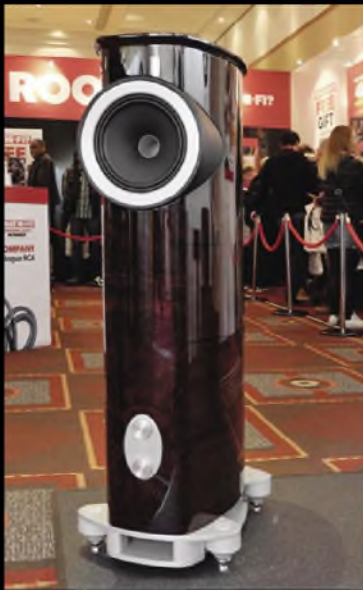
A Fyne Audio F10 loudspeaker, featuring their new 10in Isoflare point source drive unit, where a pressure loaded tweeter fires out through the centre of the bass cone. Fyne Audio told us the heavily machined alloy bass has a Tractrix flare to distribute bass energy evenly into a room.
