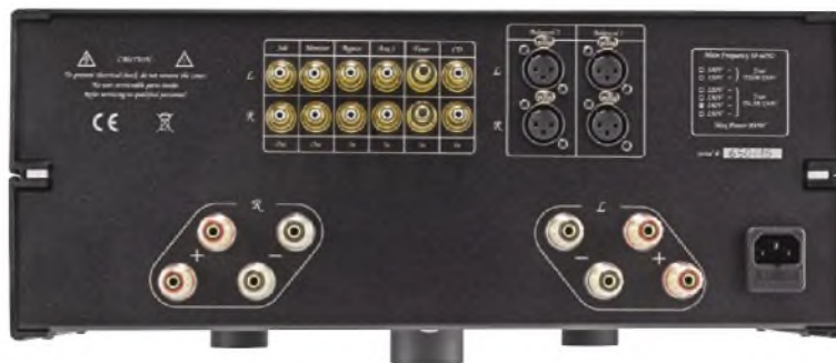
Two of the five stereo inputs are balanced XLRs, the remainder being unbalanced phonos. There's no phono stage but Unison makes provision for an active subwoofer, line-level output and preamp-skipping 'bypass' input. Two pairs of speaker terminals are provided for bi-wiring purposes.
