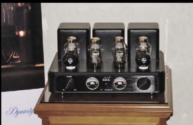
Ming-Da MC368-B SE amplifier (not the MC386-B but a variant) with onion-bulb 6SN7 valves at left and right and Jinvina KT90s at rear, presumably in parallel pairs as this is a Single-Ended amplifier. The idea here is to offer useful output power from a Single-Ended design, 25-30 Watts from parallel KT90s I'd guess.
