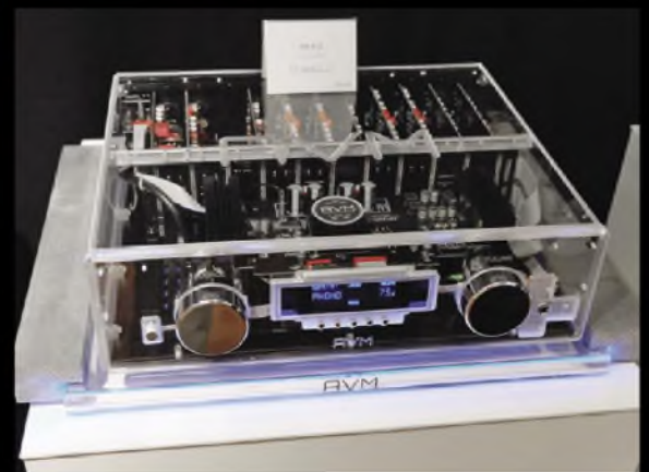
This AVM Ovation FA8.2 modular analogue preamplifier caught my eye, with its clear acrylic casing. Unfortunately, this is a show demonstrator only, designed to capture attention – and it worked! PMC act as distributors for the German brand; the product has aluminium bodywork with a tinted top window in commercial form, with a range of plug-in cards to tailor functionality.
