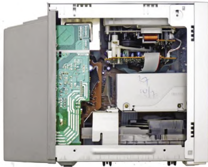
Much is crammed into the diminutive system-unit – cassette deck (top) CD transport (bottom), Minidisc (the screened box in the middle), USB DAC, FM/AM tuner, four amplifiers, system control and common power supply.
