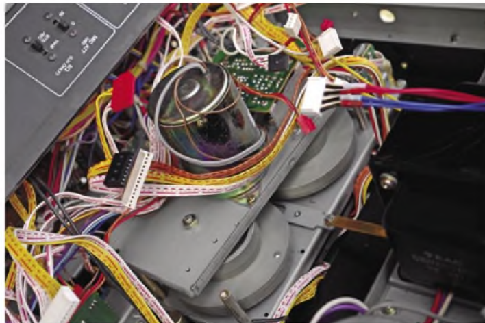
The partially dismantled capstan assembly, less belts.
