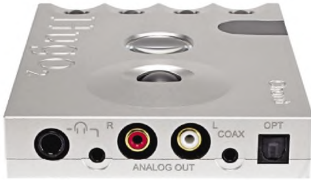
The Hugo has 3.5mm and 6.3mm headphone sockets, plus analogue output and coaxial and optical digital inputs.
