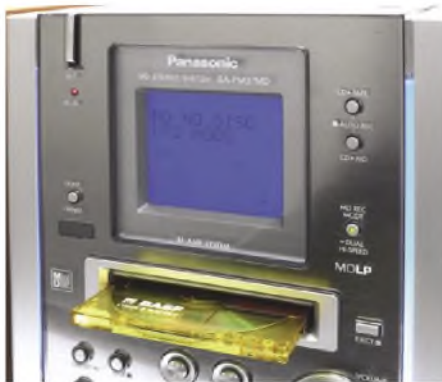
The slot-loading Minidisc feature is one of the PM37MD's high points – its recordings are audibly-superior to those of the cassette deck.
