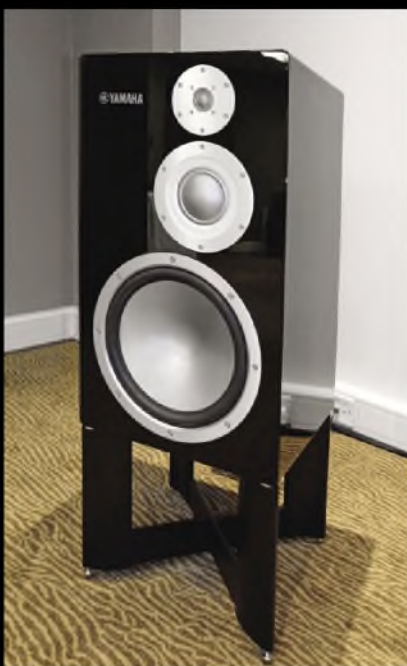
Here's a loudspeaker to catch the eye: Yamaha's new NS-5000, a spiritual successor to their much admired NS-1000M that used a beryllium midrange dome drive unit. The NS-5000 uses Zylon synthetic fibre domes coated with a 'Monel' alloy, Yamaha say, to avoid the resonances domes commonly suffer. They are accompanied by a 12in bass unit, just as before. Impressive!
