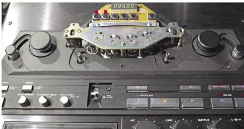
Teac-x2000m. The head plate that has to be removed for access
