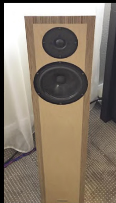
New UK company 3 Square Audio had a pair of its Translator floorstanders on demonstration. They are constructed using bespoke Birchwood cabinets and employ a first order crossover. At £2800 they sounded very smooth and refined.
