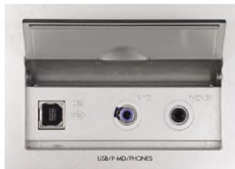
What makes the PM37MD special – and arguably still relevant today – is the USB input, which still works with up-to-date operating systems like Windows 10. Thanks to this, something that turns up cheaply at car-boot sales can be pressed into service as a compact audio system for the PC in your office or study.
