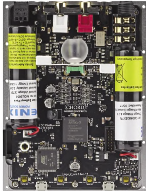
Internals are neat and tidy with (centre) Chord's own DAC circuit designed by Rob Watts.
