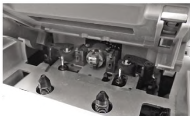
The PM37MD's auto-reverse cassette deck transport. The head-stack revolves into the position appropriate to direction.
