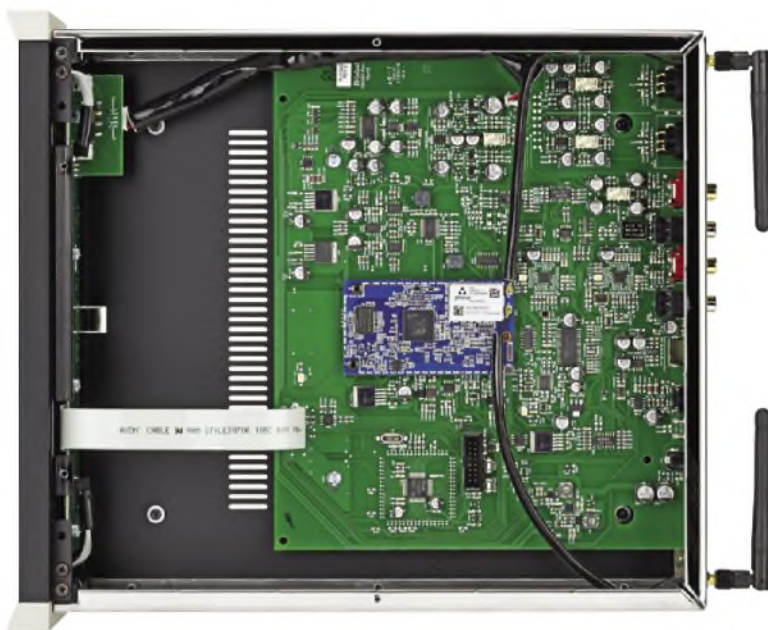
The neatly laid-out circuitry of the McIntosh MB50. Note the two wi-fi antenna on the rear for a more stable network connection.
