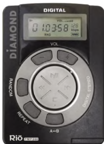
The basic controls of the PMP300 – they're closer to what you'll find on a CD player than one of today's touchscreen marvels. The simple LCD screen is incapable of showing the name of the currently-playing track, but it will reveal its MP3 bitrate (here, 128kbps).
