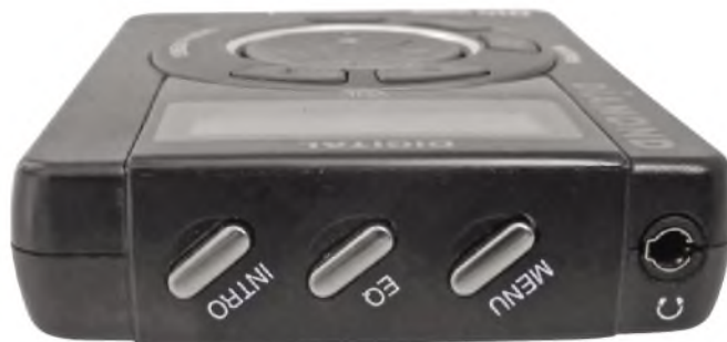
The PMP300's top panel. An equaliser – with 'jazz', 'rock' and 'clas(s)ic' presets, plus normal' mode. All the 'menu' button does is reveal total/remaining internal/external memory capacity and the internal software version.
