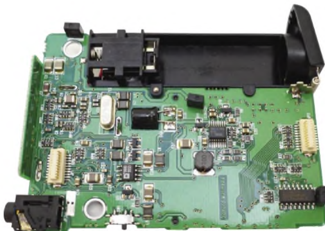
One of the two internal circuit boards of the PMP300. This one contains the power supply electronics (including the DC-DC converter) and the analogue circuitry (such as the headphone amplifier).
