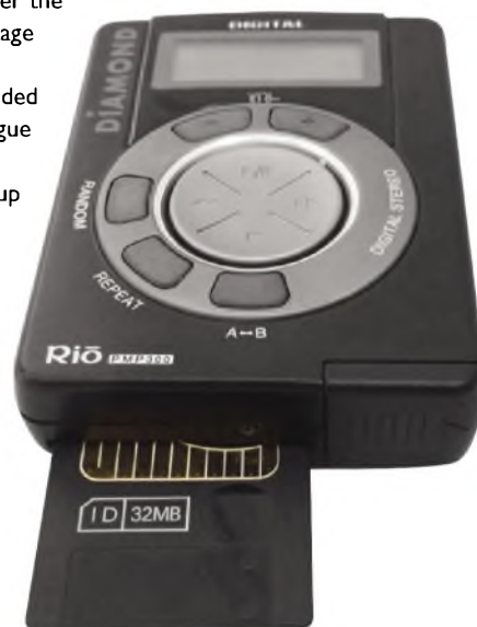
The use of flash-memory reduced power consumption, made players impervious to shock and provided instantaneous track access – which must have impressed CD and cassette listeners. But the era's technology had its limitations. The PMP300 alas offered a mere 32 Megabytes (MB), or around 0.03GB.
