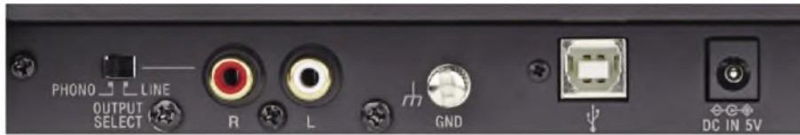
The rear panel has a small Phono / Line output switch that selects the phono stage, or bypasses it. There are analogue outputs, an earth terminal, a USB output for a computer and a 5V power supply input.
