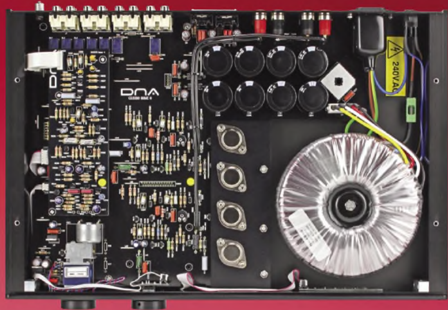
A classic design, implemented with modern components and production techniques. Note the four metal-cased power transistors of the output stage, which are to the left of the toroidal mains transformer. Above the motorised volume control can be seen the phono stage.
