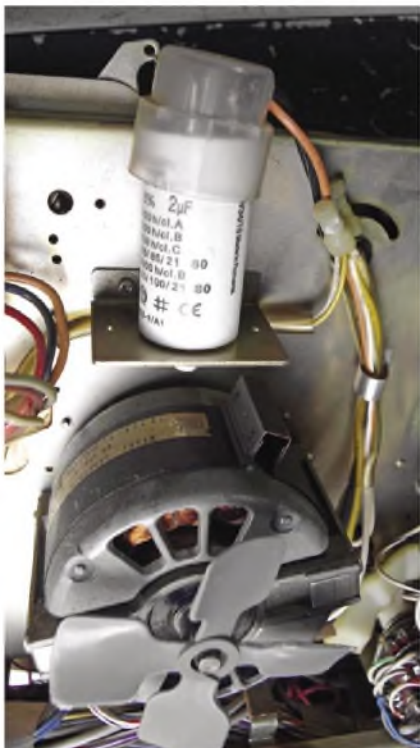
The motor run capacitor (polyprop). The original is a 1.5µF+0.5µF so 2µF is fine as a replacement.
