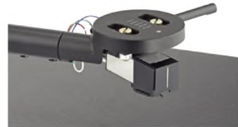
The fitted cartridge is budget design with V magnets and is similar to an Audio Technica AT-95, but with conical stylus and 3g tracking force. Yet it is made in China for Sony and only a Sony replacement stylus can be used. Note the fixed headshell.
