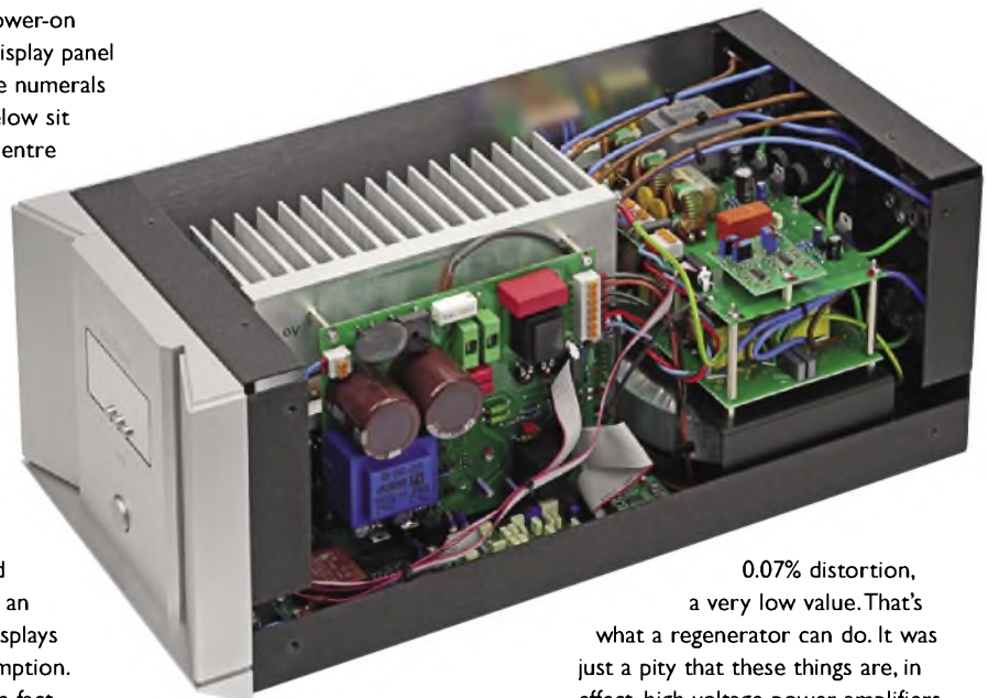
A complex interior with large heatsink of the 150 Watt high voltage amplifier dominating.
