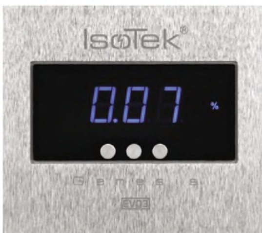
Mains input distortion of 4.58% (top) and mains output distortion of 0.07% (bottom). These were our conditions; both values can vary.
