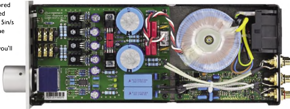
Internal construction is impeccable. Note the hefty power supply, and the heatsinked power transistors that form part of the headphone output stage. The amplifier/power supply board dwarfs the DAC, which can be seen under the toroidal mains transformer; despite their proximity, no untoward effect on sound quality was evident.
