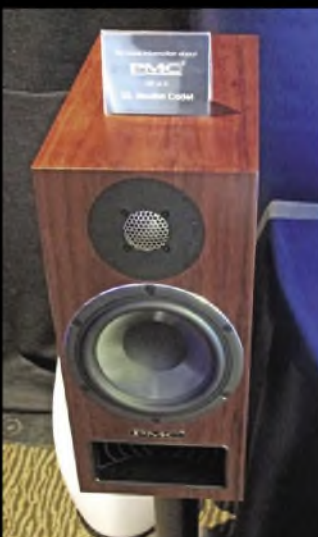
Loudspeaker manufacturer PMC celebrated its 25th anniversary by showing its new twenty5 series. The models include a new Laminar vent design and the company's most advanced Transmission Line technology.
