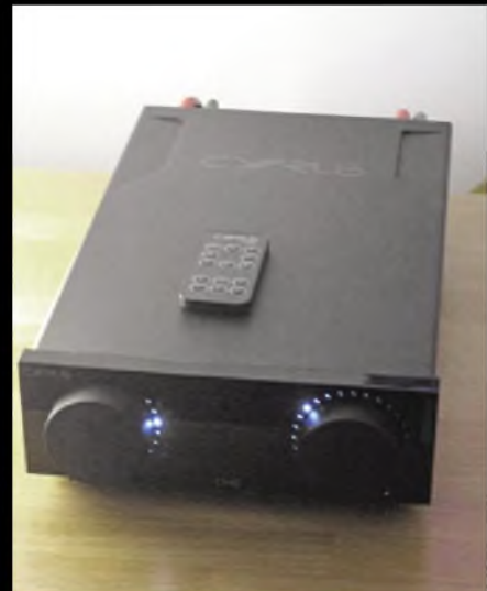
Also breaking cover was the Cyrus One - a new integrated amplifier featuring the company's latest 3rd generation Class D circuit and producing 2 x 100W of power, Bluetooth connection, a dedicated class A/B headphone amplifier and an MM phono-stage.
