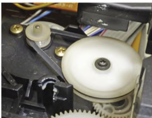
The lasers, motors and electronics of Pioneer players are resilient but belts can stretch causing the pulleys to slip. Replacements are readily-available.
