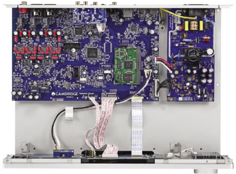
Cambridge also takes pride in the internal layouts of its products. The CXN's analogue electronics – note the two Wolfson DAC chips, high-quality capacitors and muting relays – is at the opposite end of the enclosure to the switch-mode power supply. The green sub-board is the Zander streaming module.
