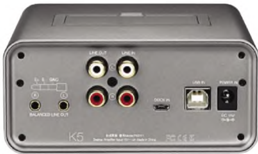
The K5's rear carries balanced outputs through three-pole 3.5mm jack sockets, rather than XLR sockets. There are digital pass-through inputs and connector for an external power supply, as well as Line inputs/outputs.
