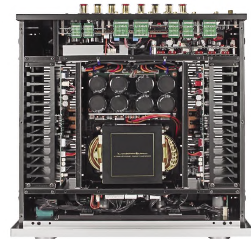
Internally, the Luxman L-590AX MkII demonstrates this company's immaculate build quality and attention to detail. At lower centre is the mains transformer and above it rows of circular smoothing capacitors of the power supply. At left and right are large heatsinks to keep the output transistors cool under Class A operation.
