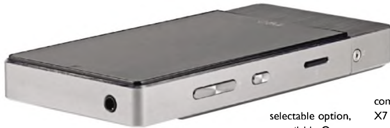
This top view shows the Line/Coax (digital) 3.5mm four pole output jack. The left side has volume, on/off buttons and a microSD card slot.
