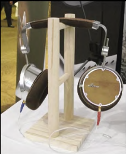
Far East based oBravo was displaying its innovative HAMT-1 over-ear headphones. A truly luxurious model they feature an Air Motion Transformer tweeter allied to dynamic neodymium midrange/bass drivers. They didn't just sound good - they looked good too with a handsome wood finish.
