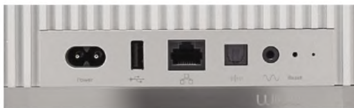
Inputs include USB, optical digital, ethernet as well as 3.5mm analogue line-in.
