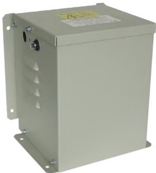
RS Components sell a Carroll & Meynell 1.65kVA fixed, encased transformer for 'garage use' that can deliver 15A from twin centre tapped 110V secondaries (Part No CM 3300 WMO, price £296.75). It must be wired in by an electrician. Downloadable safety instructions provide detail.
