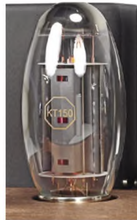
The gherkin-shaped Tung-Sol KT150 Russian-made valve offers exceptional power for a single-ended design.
