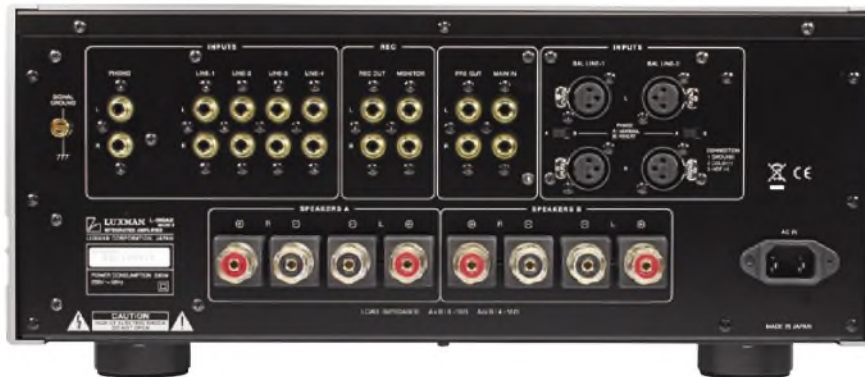
The rear panel of the Luxman shows the range of inputs available - balanced XLR sockets at right, plus unbalanced RCAs including a single switched MM/MC input at far left. Gold plated speaker terminals accept bare wires, spades and 4mm banana plugs.
