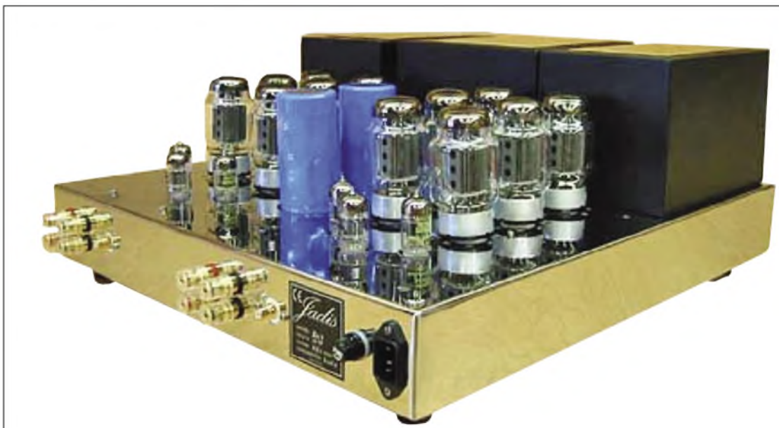
A Jadis Defy 7 amplifier: three banks of KT88s working in push-pull pairs giving 60 Watts in Triode mode, in Geoff Wilton's system. But why does this amplifier now hum, asks Geoff?
