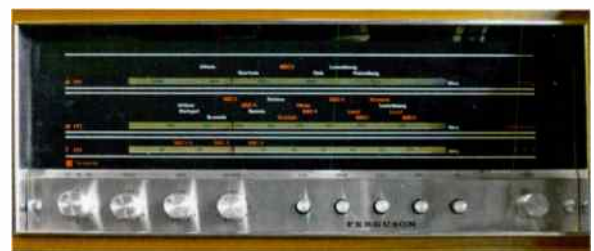
The receiver of the Ferguson 3361 has a late 1960s/early 1970s look. It's easy to use – bass, treble, balance, volume and tuning knobs – plus selectors for tape, gram, VHF/FM, MW and LW.
