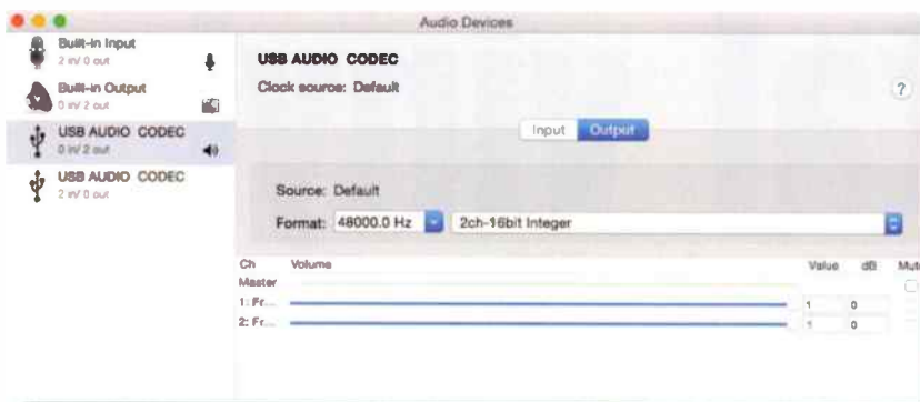
This is the AudioMIDI sound panel of a Mac, buried in a Utilities folder in the Applications folder. Go here to set digital options such as bit depth and sample rate.
