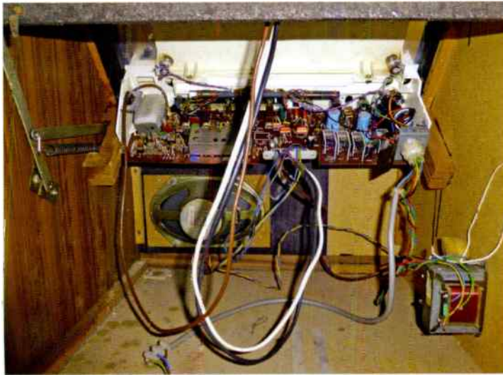
The 3361's receiver board in the stereogram cabinet. The wiring, mains transformer and right-hand speaker are visible.
