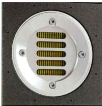
The folded ribbon tweeter comes from German manufacturer ELAC.
