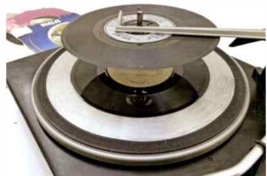
Here the Garrard 2025TC changer has been removed from the 3361 for servicing, and is now undergoing final tests. In this picture, records (in this case, 7" pop singles) are loaded for sequential playback. All records played in this mode have to be of the same size and speed – mixtures aren't possible. The 2025TC's 'manual' mode is of course much kinder to records.
