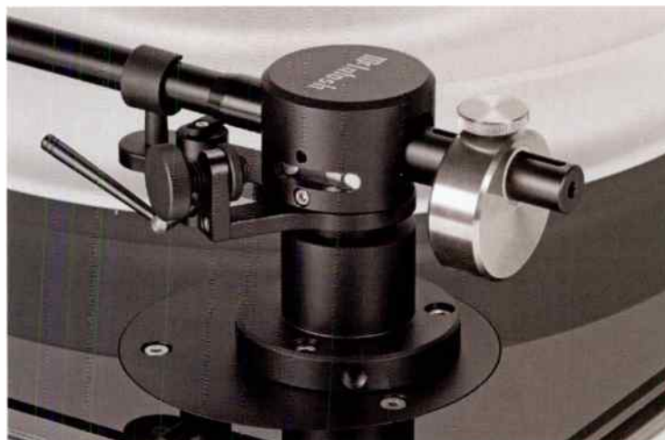
A large knurled-edge thumbwheel at left applies magnetic bias correction to the arm. The rear counterweight is uncalibrated so a stylus downforce gauge is needed.
