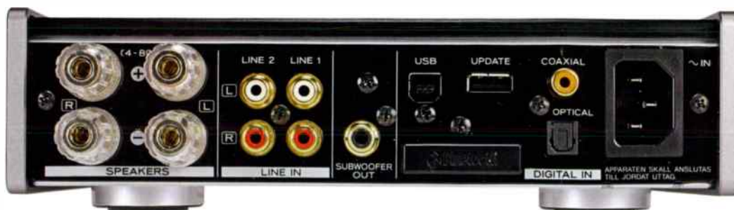
A good selection of inputs and outputs that cover analogue, digital and 'smart' sources. Note how the speaker terminals, which will accept banana plugs or bare wire, dwarf all else in this small case. The integrated Bluetooth aerial can be seen bottom right.
