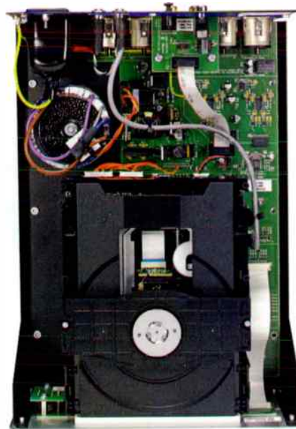
Inside the Leema Elements uses a tray-loading CD mechanism and the company's latest Quattro-Infinity DAC technology.
