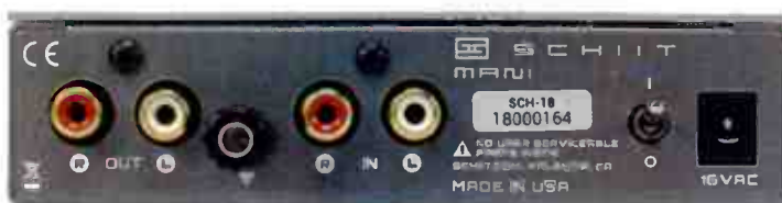
The usual phono amp connections are available. Nice to see a firm, decisive toggled power switch (right).
