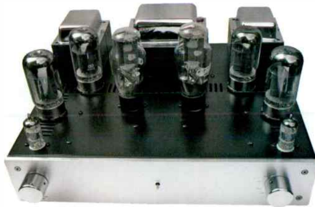
WAD 6550 valve amplifier produces 40W per channel but "runs out of steam quickly" in a big room, says Anthony Parkin.
