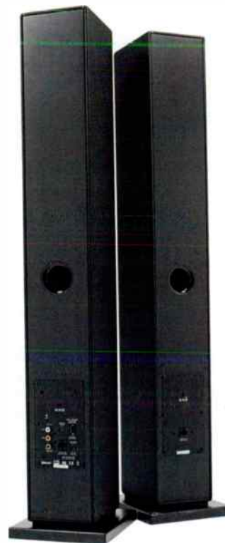
The rear of the master speaker (left) features a pair of RCA analogue inputs, an optical digital connection and a subwoofer output for those wanting more bass.
