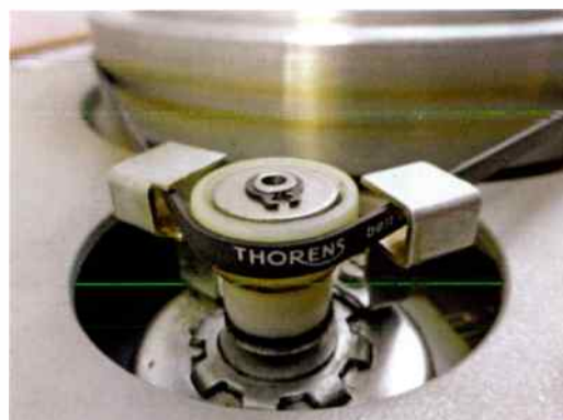
The TD125's sub-platter is driven via a precision-ground belt from a 16-pole synchronous motor driven by a variable low-frequency oscillator. Note that in the Mark 2 version shown here the motor pulley contains a clutch - near its base, you can see the felt pad that forms part of its design.
