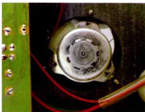
This is the powerhouse of the TD125, a synchronous AC motor. For later versions of its replacement, the TD126, Thorens was to move to a DC motor with servo speed control. Thorens had obviously learnt from its mistakes; the TD126's 78rpm speed is more useful than its predecessor's 16rpm. The TD125 can, however, be modified to play 78s.
