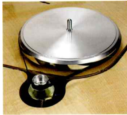
The belt-drive mechanism sits inside a completely rebuilt plinth assembly.
