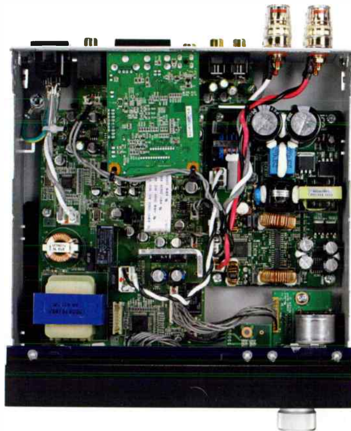
A rather busy interior! Thanks to efficient Class D amplification, less power is wasted so there's no need for massive heatsinks. Note the motorised volume control (bottom right) and USB interface PCB (top).
