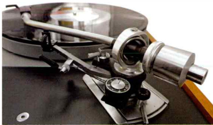
Seen by some as a 'poor man's' alternative to the ubiquitous SME 3009 S2, the Japanese-made Acos Lustre GST-1 is of a completely different design. Dating back to the early 1970s, this nicely-made S-shaped tonearm still works well with compatible cartridges (typically high-compliance MM designs). Its features include removable headshell, magnetic bias-compensation and, by the standards of the time, user-friendly setup.
