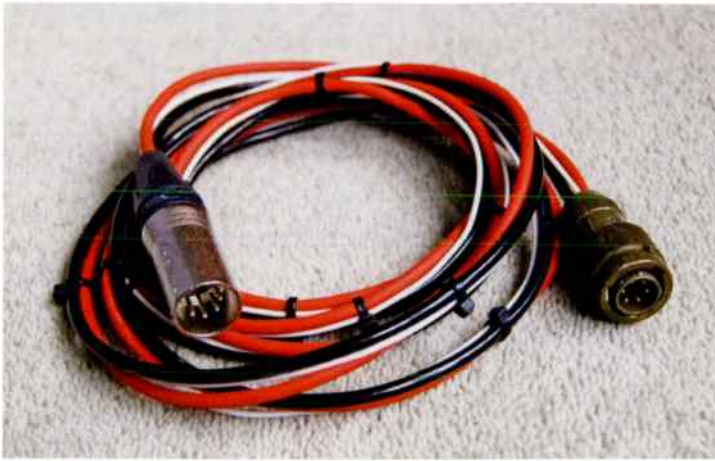
Fig 1 - A lead made by David Lord with XLR at one end (left) and Amphenol 62GB at the other (right).
