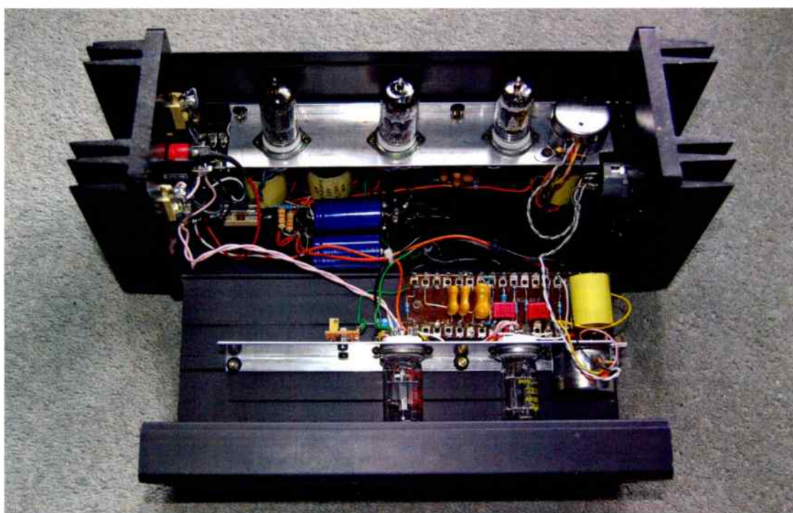
Fig 5 - Sowter Model No 1990 MC transformers in the preamp chassis – tubular screening cans at right.
