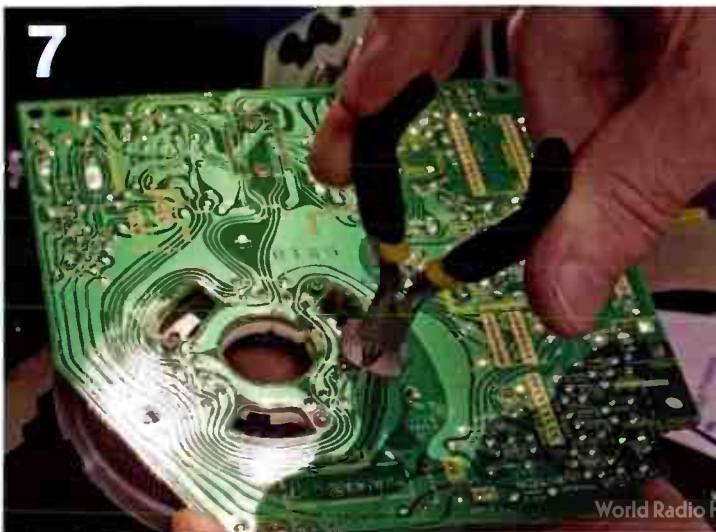
▲ With board and motor screws removed the combined board/motor assembly can be lifted out. This then reveals the main bearing that is to be replaced.
