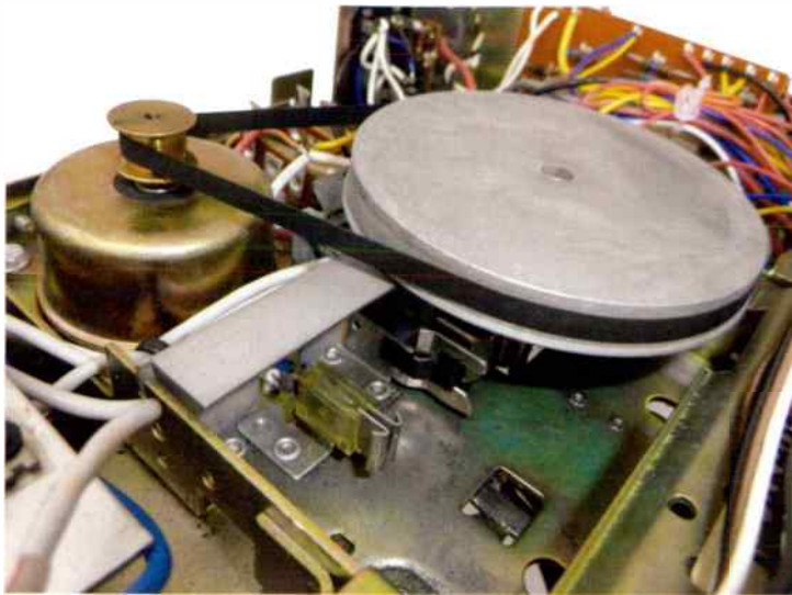
Inside, eight-track players are somewhat basic - the mechanism was clearly designed to be as cheap and reliable as possible! The capstan's massive flywheel is coupled to the motor via a flat drive belt. To facilitate a simple 'fast forward' function, the motor is run at a higher speed (during this mode, the audio circuits are muted to prevent 'monkey chatter')
