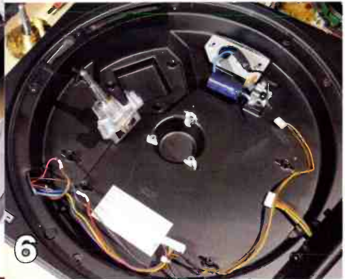
▲ The main bearing is free to be lifted out. The Mike New bearing then drops into its place. It must be aligned with tapped lugs in the chassis, using the long motor screws, before the board/motor assembly is replaced.
