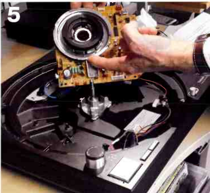
▲ With board and motor screws removed the combined board/motor assembly can be lifted out. This then reveals the main bearing that is to be replaced.
