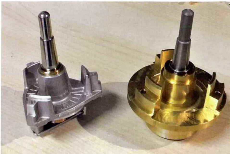
At left the original Technics bearing, at right its replacement.
