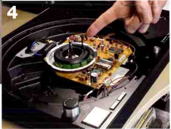
▲ Three screws holding the board to the chassis must be removed, then another three holding the motor assembly down to the chassis; they pass through the bearing assembly and hold it in place too.
