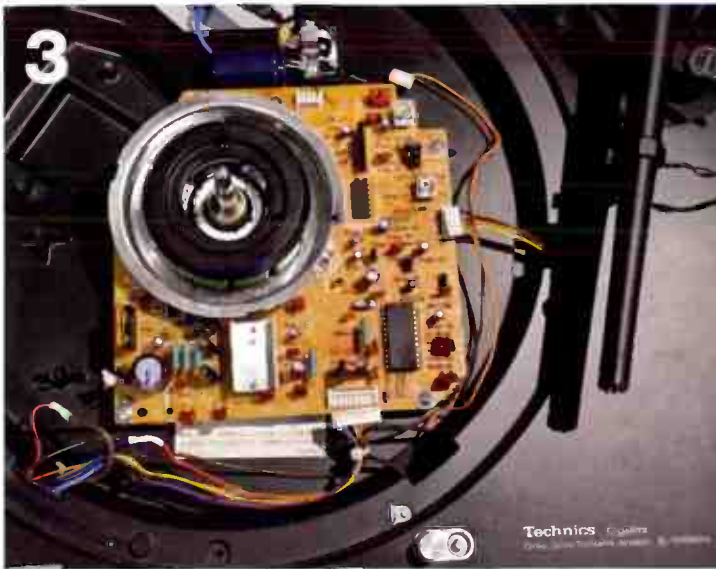
▲ The circuit board has three white, multi-pin connector blocks. These must be disconnected, preferably by easing them apart with a small jewellers' screwdriver, rather than pulling on the wires. There are no spring clips; they are a simple friction fit and slide apart.
