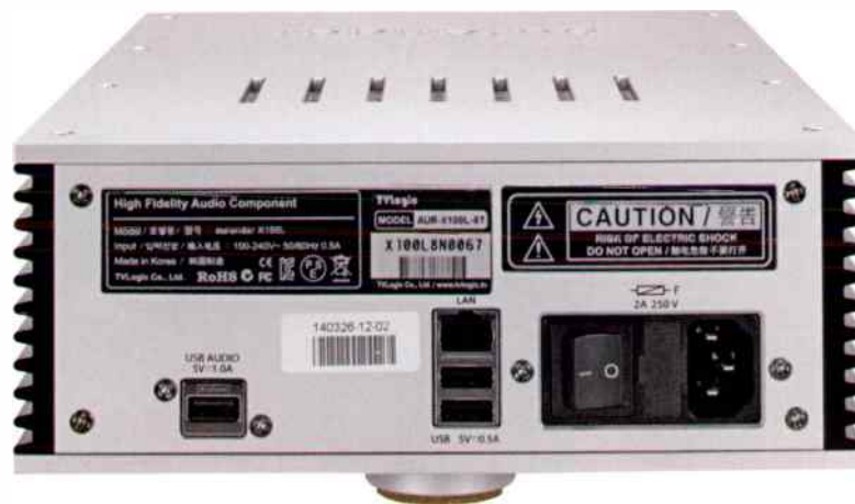
The rear view is uncluttered. There is no S/PDIF output, only USB.
