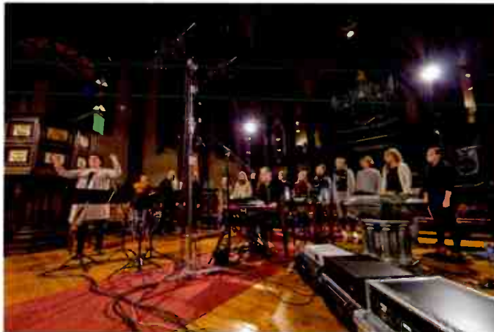
Modern recordings are now a long way from mono or stereo; here is 2L of Norway recording with "9.1 DPA microphones array, in DXD (352.8kHz/24bit)" at Uranienborg church, Norway.
