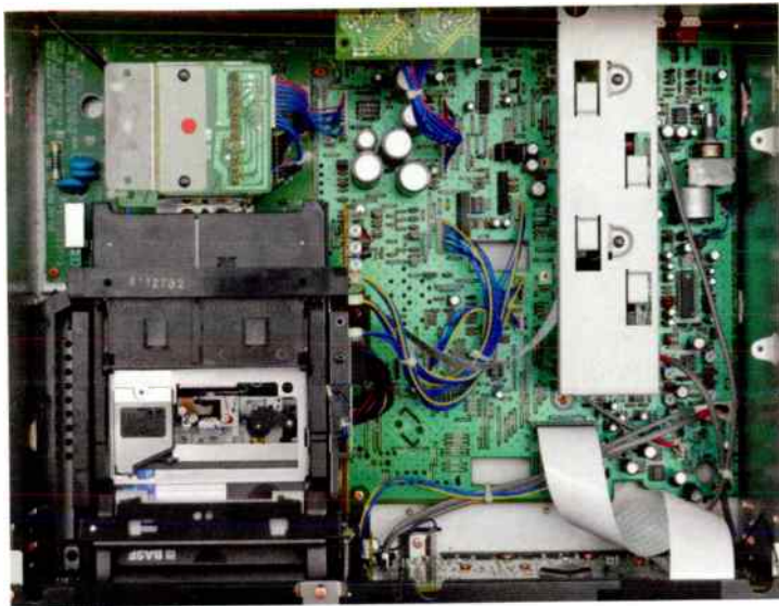
Here we have the neat internal construction of the Marantz DD82. To the left can be seen the tape transport; to the right the motorised analogue output-level potentiometer. Next to the latter are the vertically-mounted digital-audio and PASC compression boards.
