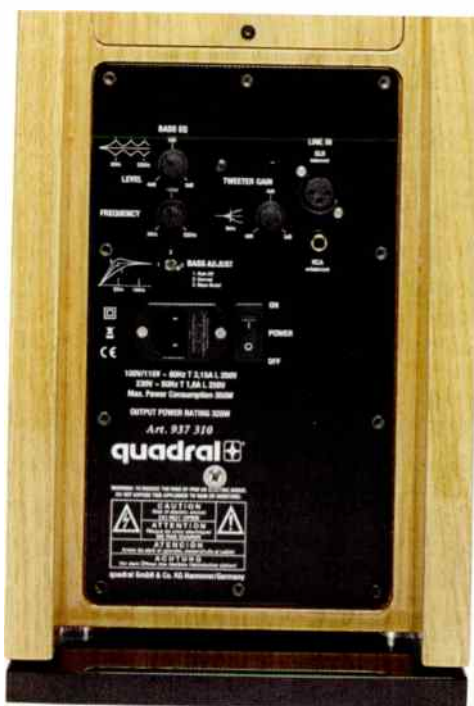
At top left is Band EQ, a parametric equaliser, with frequency and level (+/-6dB) adjustment knobs. Below, is a Bass level three-way switch. To its right is a Treble level adjustment knob.
