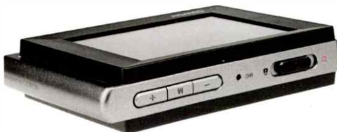
Volume up and down buttons and a microphone are placed on one face, plus a power switch.
