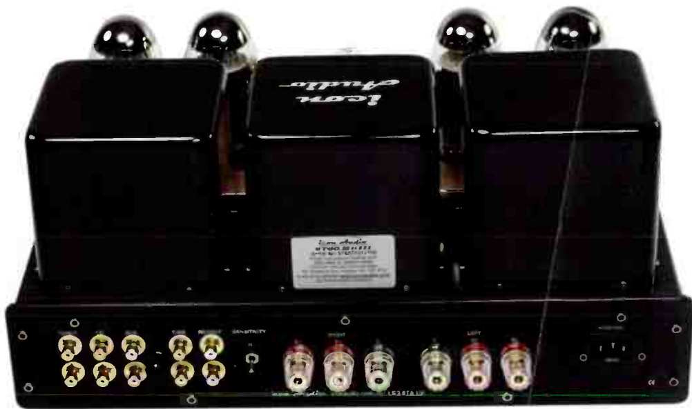
Loudspeaker output terminals are gold plated and fully shrouded, catering for 4 Ohm and 8 Ohm loudspeakers. The sensitivity switch sits between them and the inputs.
