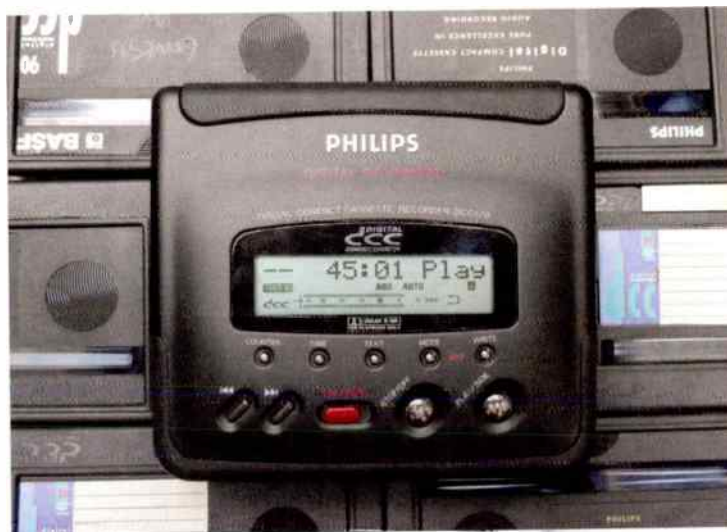
The compact Philips DCC170. Save for a Marantz professional machine, it was the only portable DCC recorder sold in the UK. An excellent playback device, it was limited as a field recorder by relatively-limited recording time and rather noisy microphone preamps.
