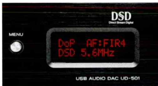
The Teac's DSD display shows DoP transmission protocol, Audio Filter FIR4 selected and a double rate file (5.6MHz) being played.
