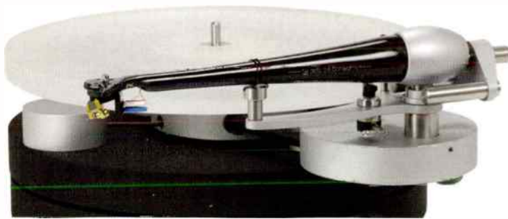
The rear counterweight along the axis to set tracking force and around it to adjust lateral balance.
