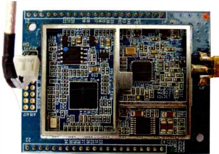
A close-up view of the Gyro module, which provides all tuner functions. In FM mode, it works very differently to conventional tuners.
