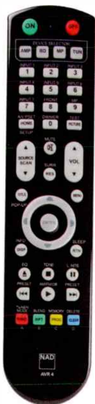
The remote control possesses loudspeaker load settings, and room bass equalisation that must be adjusted at the seating position.
