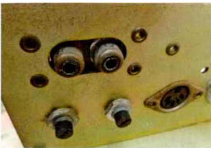
Conventional phonos and a DIN socket yield the audio output, complete with level-matching 'pots'. The phono sockets tend to rust, and alternative arrangements are recommended.
