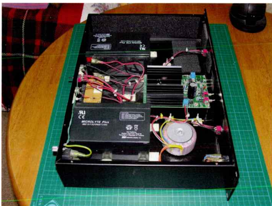
The 12V lead acid battery power supply, with mains charger, built by Peter Graves. It "opens out the sound" he says, "adds more detail and depth and firmer bass".
