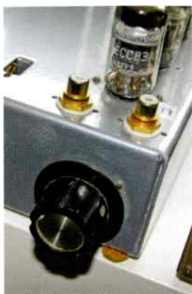
Volume control fitted instead of pre amp socket.
