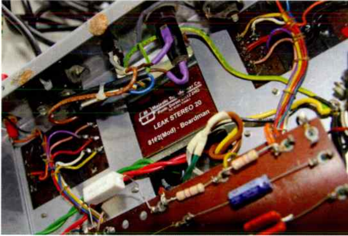
Famous 3 watt resistor - do not increase the value.
