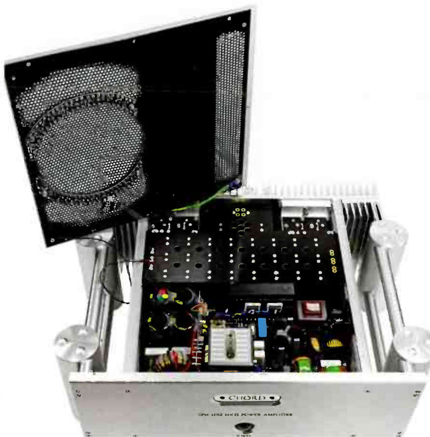
Inside the Chord - a bespoke SMPS power supply.
