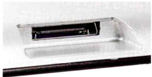
The multi-pin connector carries USB, charging and HDMI via an adaptor.
