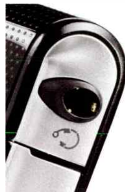
A 3.5mm headphone jack carries analogue audio only; there is no optical digital output. An SD memory card can be loaded too.
