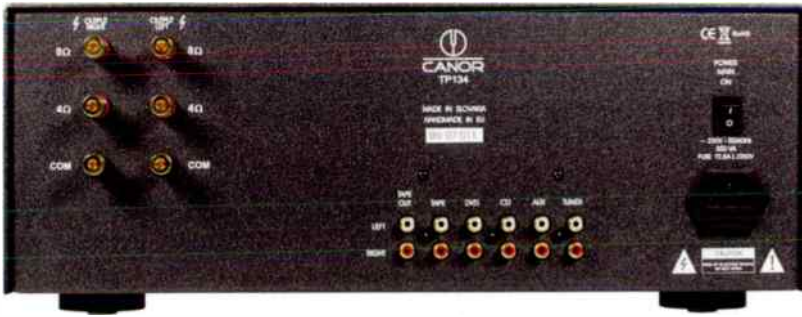
8 Ohm loudspeaker outputs with 4 Ohm taps are fitted, connection being through gold plated 4mm terminals.
