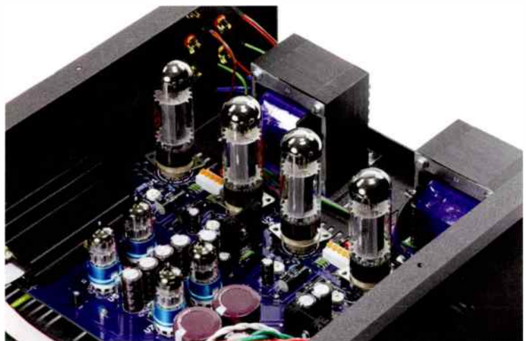
The amplifier has an electronic management circuit to control switch-on, biasing and other functions. Remote control is provided.
