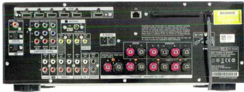
A wi-fi aerial and ethernet socket (top right) provide network connection.
