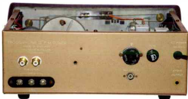
Rear view of Trough-Line showing stereo sockets fitted
