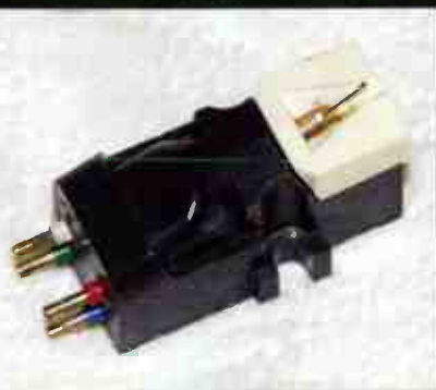
Miracle transformation; lowly Goldring MM fitted with new cantilever and stylus.
