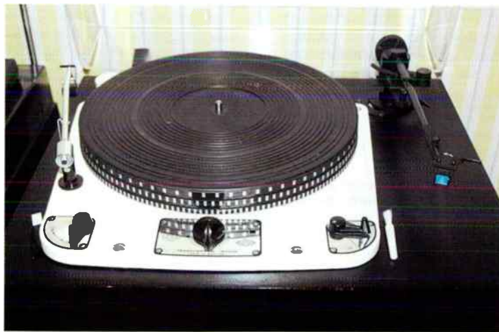
A Garrard 301 deserves a good matching arm and cartridge. It may be a golden oldie but a modern arm best suits.
