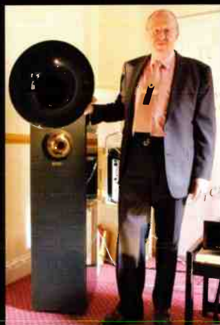
A German Acapella horn with its astonishing plasma tweeter. This isn't the same tweeter used by Lansche, we were told, but their own unique design. NK
