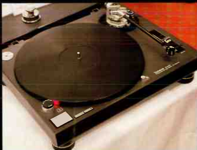
Spot the difference! This Technics SL-1210 turntable is missing its strobe markings. That's because the new platter is custom made to be less resonant than the original mazak casting, so adding less to the sound. NK
