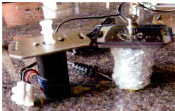
The new OL DC 200 motor left, with the old (sound proofed) unit on the right.
