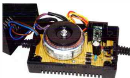
Inside view of the new receiver power supply fitted with the Fidelity Audio Spower voltage regulator.
