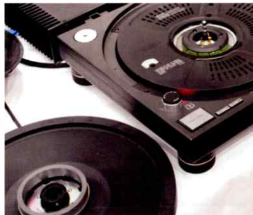
Technics used their own Linear motor within the SL-1200 turntable, with rotor magnets in the platter, seen here.
