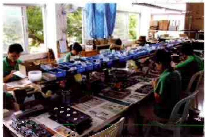
Valve amplifier production at Mei Xing is manual - all components are placed at right angles, with bare earth bus bars and neat wiring looms...
