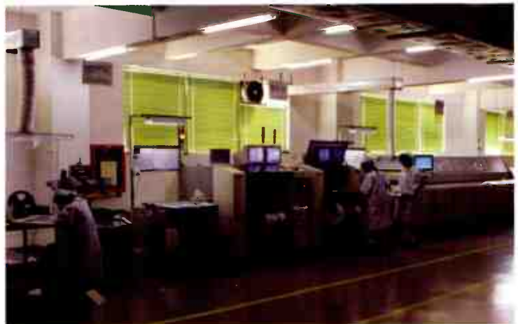
Surface Mount component placement machines at IAG carry out fully automated board assembly using miniature components.
