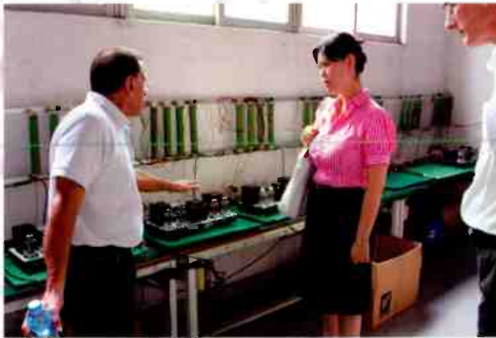
Lux valve amps soak test in one of IAG's many test rooms where products are run and tested. Mr Ali (left) explains the procedure to Anna Chang of Hi-Fi World, whilst Peter Comeau looks on...
