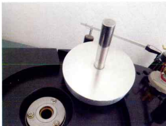
The 20mm diameter main bearing and machined alloy subplatter...
