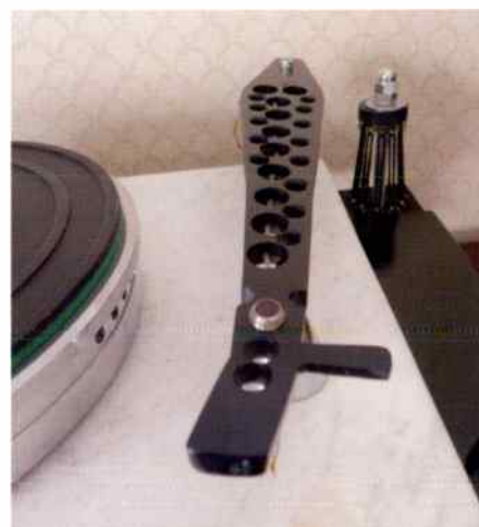
The arm of RC23 is made of Perspex and sits on a hardened steel spike which rests in a micro-ball race.
