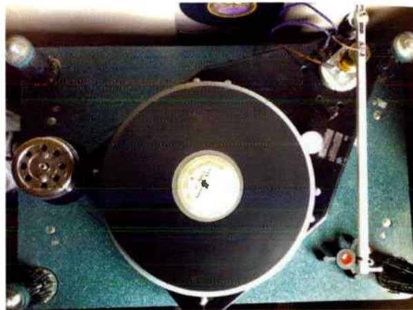
The lead loaded motor housing passes through a hole in the top plinth and is mounted on the lower plinth.
