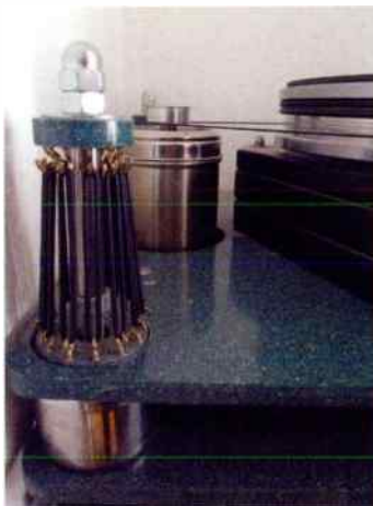
The shaft in the middle of the rubber bands sits in a pot of STP oil, mounted on the lower plinth...
