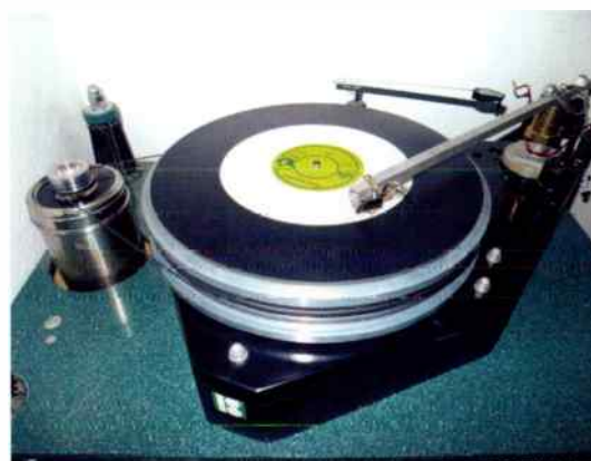
The main bearing and the arm are mounted in three layers of slate which total 80mm thick!
