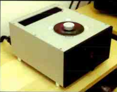
The German AcousticPlan Vadi CD player, imported by GT Audio, has special analogue filtering and valve output stages with balanced output using audio transformers, all to achieve a more natural sound than is usual from CD. NK
