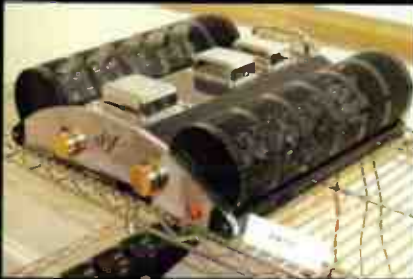
Tim de Paravicini told us his new EAR V12 amplifier uses six EL84 output valves per channel in parallel push-pull to deliver 50 Watts through a balanced bridge output transformer. Price is £6,550. NK
