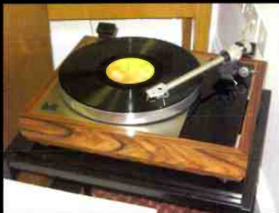
Inspire Hi-fi's Vivid LP12 kit includes a brand new real wood veneered plinth, arm board, Hercules power supply, acrylic subchassis, acrylic mat and base - fully fitted for £699. The modded Sondek sounded dramatically different to stock; tight, taut and incisive. DP
