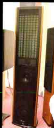
The new Kingsound Queen II hybrid electrostatic loudspeaker, imported by Icon Audio, uses an electrostatic midrange/treble panel, coupled to a box bass unit. Should be good. NK
