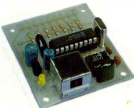
PCB mounted Infra-Red receiver and decoder module sits behind the front panel
