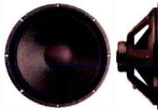
Eminence Alpha 15" driver, Fs of 41Hz and Qts of 1.26, LF sensitivity 94dB.
