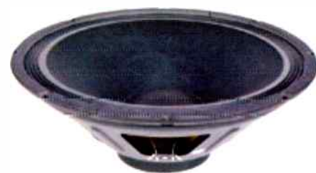
Beta-15 Eminence Beta 15" driver, Fs of 35Hz and Qts of 0.58, LF sensitivity 96dB.
