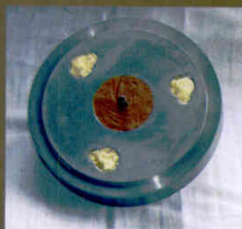
Top of TD125 hub showing infill and centre infill.
