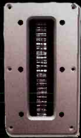
The Aurum Cantus G1 ribbon driver. Its corrugated aluminium foil carries the audio signal. It sits in a powerful static magnetic field.
