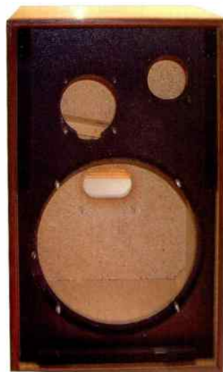
Cabinet with drive units removed.
