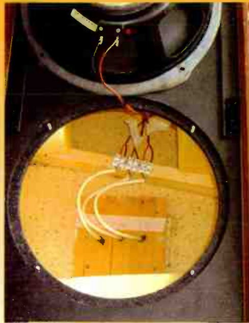
Showing cables to crossover.
