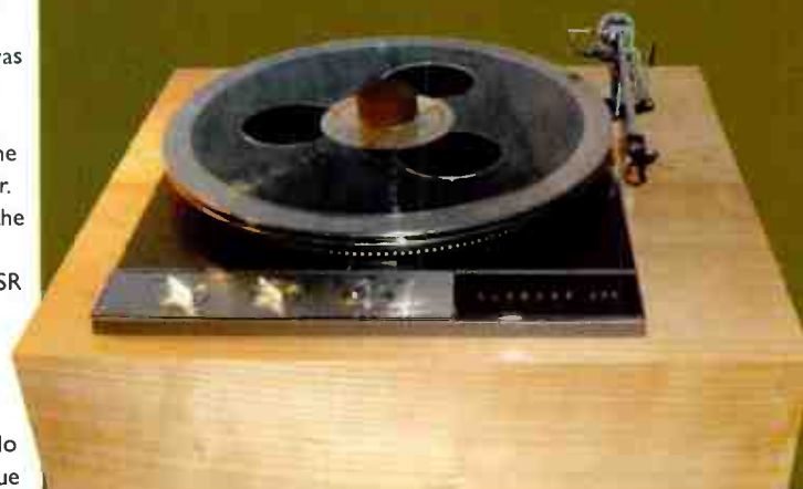
First stage: place cantering device on top of the record.
