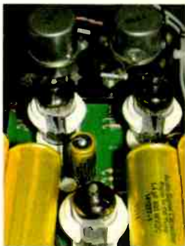
Hoops fitted to ECC83s in the Phono II.
