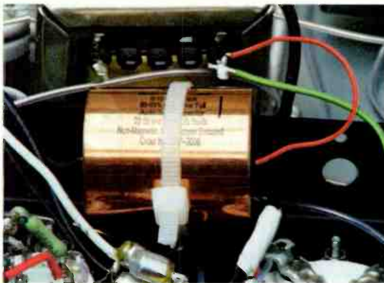
Audio Note Silver Foil capacitor fitted in place.
