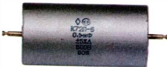
Russian Teflon capacitor.
