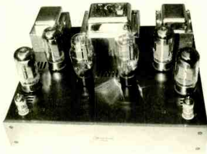
The 6550 beam tetrode gives plenty of tube power.
