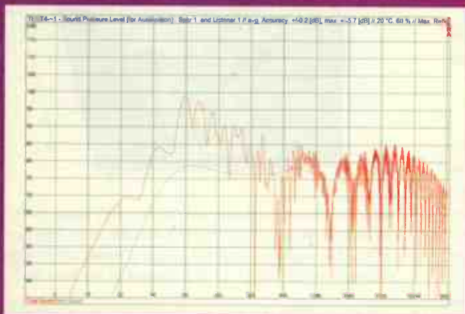
Reflections from a rear wall interfere with direct sound from a loudspeaker, resulting in reinforcement and cancellation producing a comb filter response. Cara clearly shows this effect and how well any rear surface treatment will likely reduce it.
