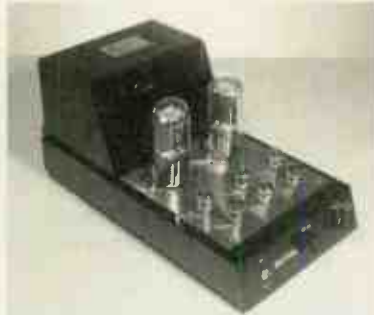
Gamma Rhythm: The 211 transmitter triode is a very popular candidate for single-ended and push-pull use.
