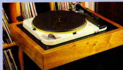
With its belt/idler drive, the 124 offers classic sound.
