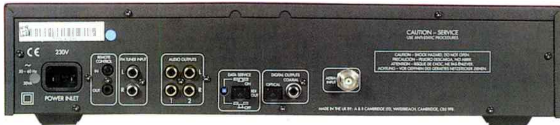
From left to right: mains inlet, remote control bus, FM tuner input, two pairs of analogue outputs, Radio Data Interface On/Off with optical output, digital outputs (coax and optical) and the single aerial input.
