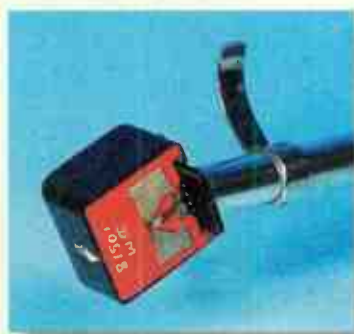
Whereas most cartridges screw onto a headshell, the Decca slides down onto a mounting plate.
