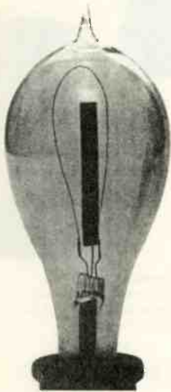
Edison inserted a plate in an electric lamp and observed that a current flowed between this plate and the positive side of the filament supply. He had invented the diode, but at the time (1883) patented it as a galvanometer. This clearly shows how the valve sprang from the electric lamp.
