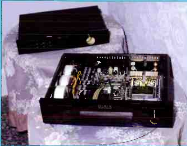
The handsome DAX converter from Audio Synthesis. The power supply consists of no fewer than three high-quality toroidal mains transformers.
