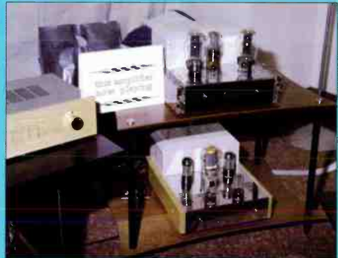
In GATE's room a 300B single-ended amplifier (bottom right hand) took its signal from the line-level pre-amp to the left which was plugged into a Leak Troughline tuner.
