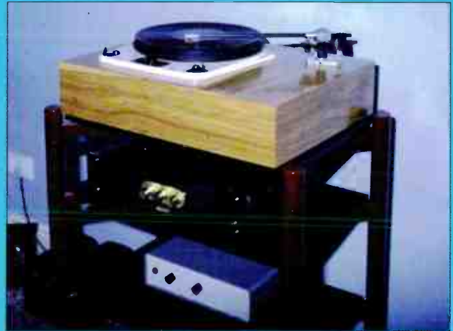
Martin Bastin's Garrard 301 was happily ensconced in his new plinth. The prototype 301/401 power supply is sitting on the rack's bottom shelf.
