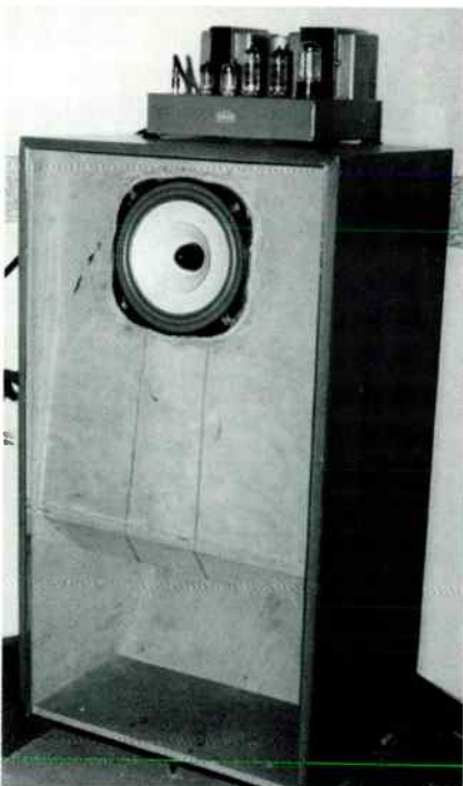
The Acousta's horn mouth is set low so that side walls and floor act to increase its area and so extend bass downwards.
