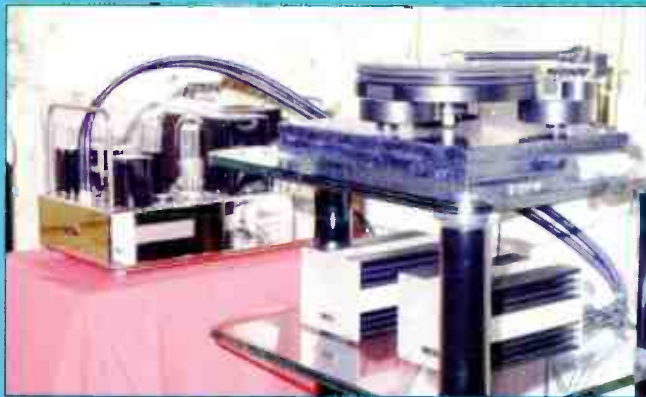
Graham Tricker's Tron valve amps. In the foreground are the line and phono pre-amps with the 211 SE amp to their right.
