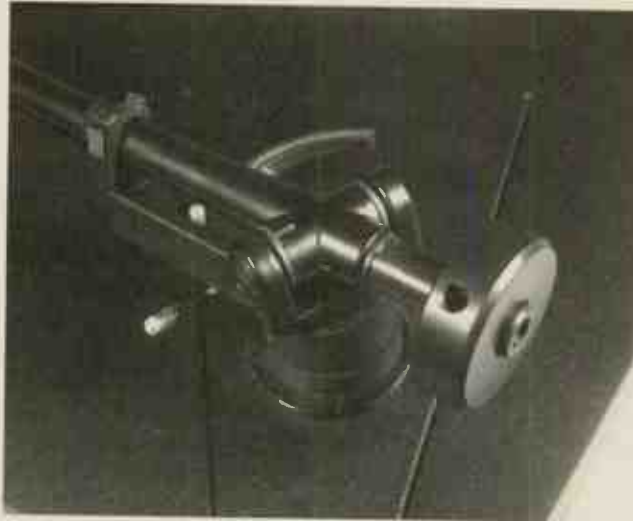
Here you can see the modification to the counterweight with its threaded hole to take the grub-screw.
