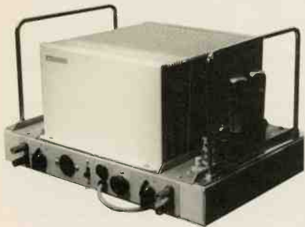
The reservoir caps in Radford's vintage STA25 power amp often fail and should be replaced with modern equivalents.
