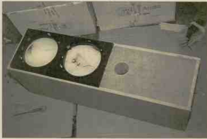
Once the baffle is securely in place, the plastic mouldings for the drivers can be fitted and the cabinet filled with wadding.
