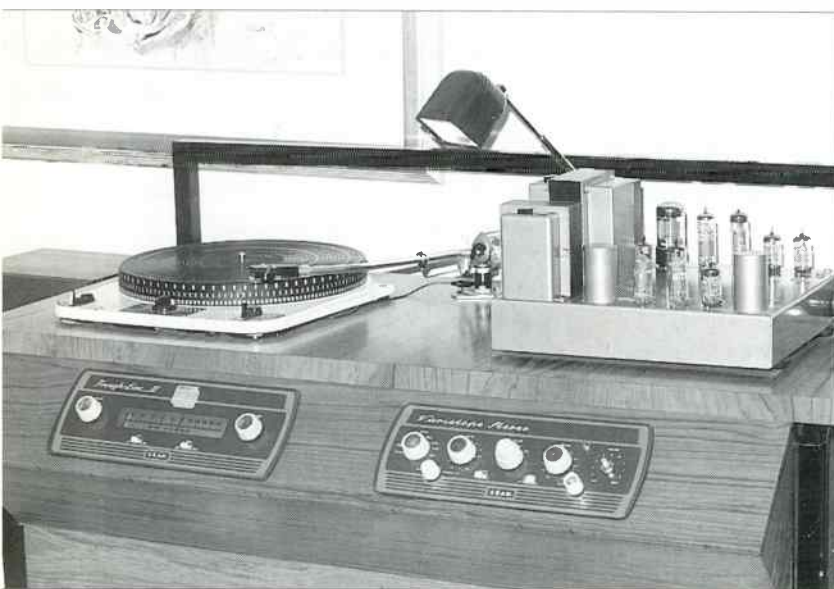
Custom console housing a BBC Garrard 301/SME3012, Leak Stereo 20 power amp, Troughline II FM tuner and Varislope stereo preamp.
