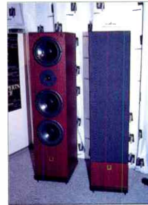
Heybrook's Heystaks use a passive bass radiator for real punch and impact.
