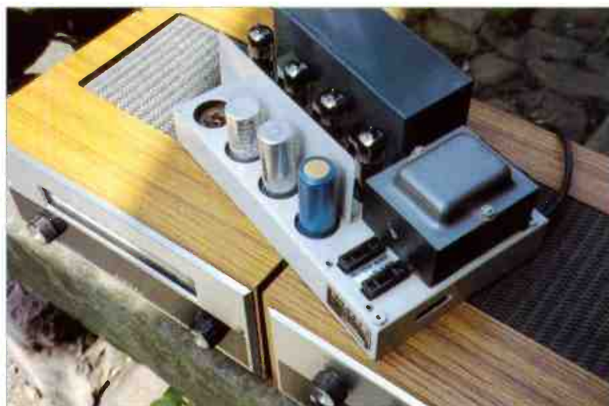
The ECL86 valves are hidden behind a metal heat screening plate to protect the smoothing capacitors.
