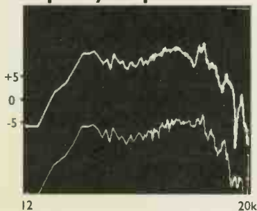
Fig 1 Above - frequency response as standard. Below - with phase plug.
