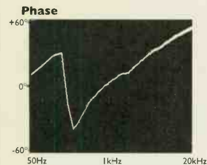
Fig 3 - Electrical V/I phase swings through resistance to capacitance above resonance, but becomes inductive again above 1kHz.
