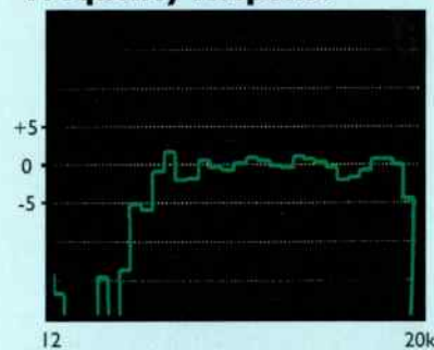
Treble falls off above 16kHz which should bring a smooth sound to CD.
