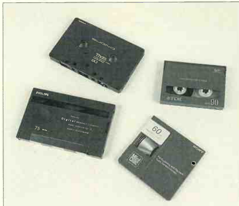
Conventional Compact Cassette (top left) is under pressure from the Digital Compact Cassette (bottom left) and MiniDisc (bottom right). DAT is used mainly for professional recording applications.
