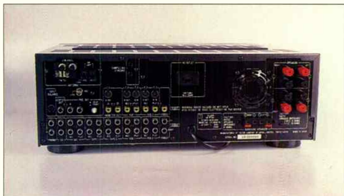
The small fan on the rear of the JVC could become audible through quiet scenes, after it had been worked hard.
