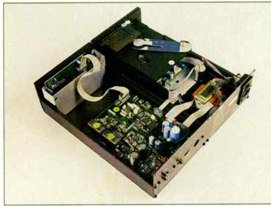
The Meridian 206ΔΣ uses two separate boxes for transport and DAC that are rigidly bolted together.
