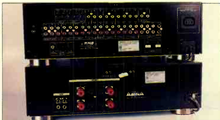
The Sony pre-amp-decoder has optical and coaxial inputs for its internal DAC. The power-amp has no output for a centre channel.
